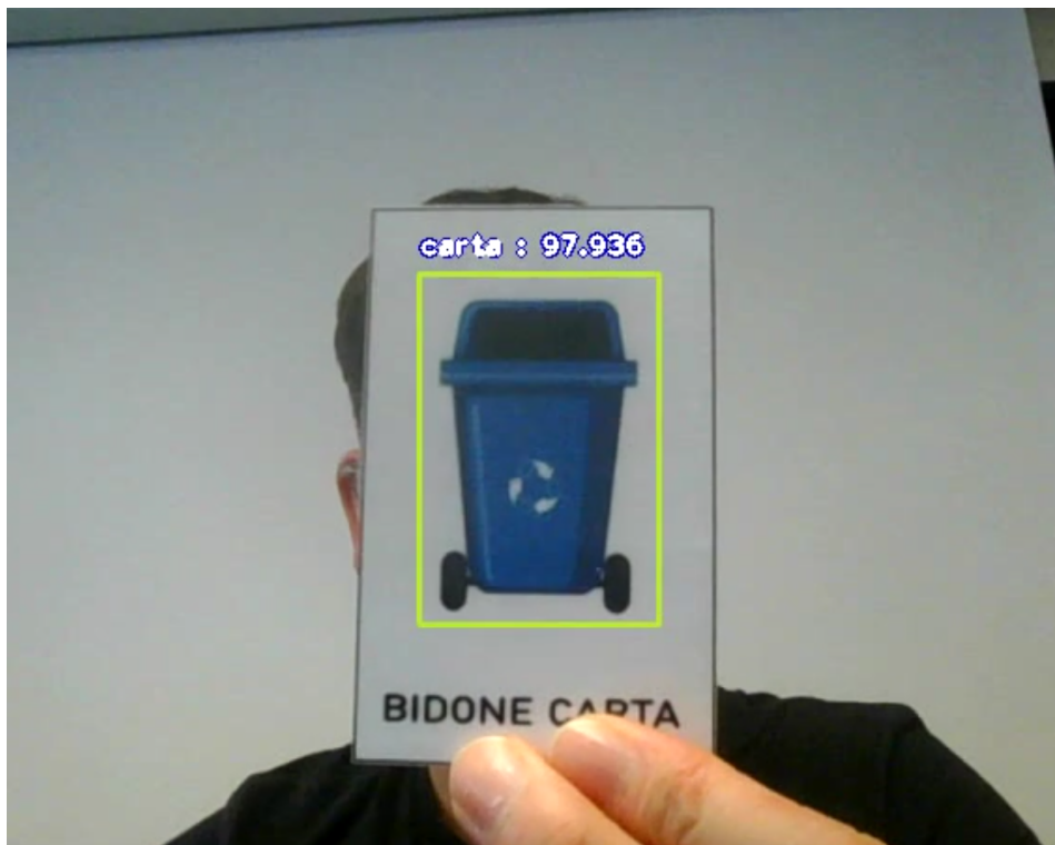
Figure 4.29: Output of one frame of the NN that recognize cards with a threshold of 0.95 .
