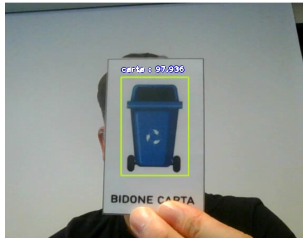
Figure 4: Output of one frame of the NN that recognize cards with a probability of 97.93% .
