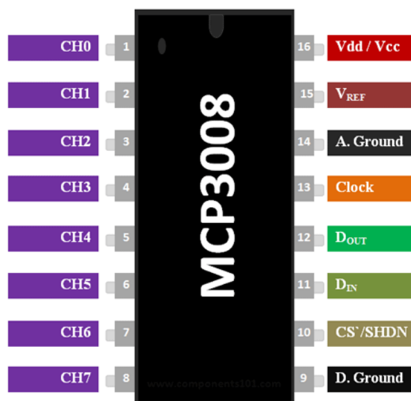
Figure 3. 15 MCP3008 Analog to Digital Converter IC – Pinout
