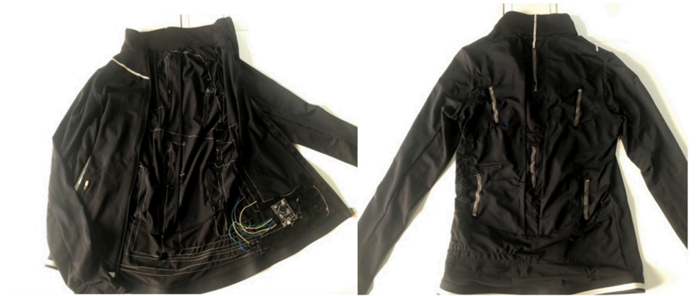
Fig 30. Prototype clothing circuit sewing inside and outside
