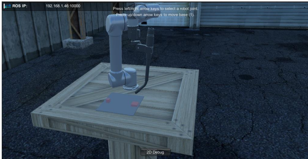
Figure 29: Completed weld with UR5 and torch 1 configuration.
