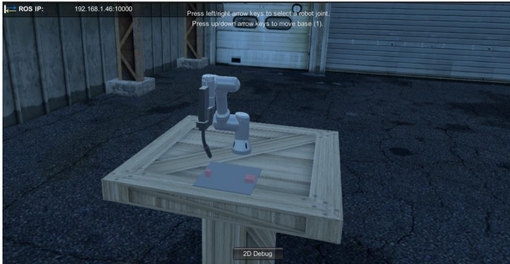
Figure 28: Welding torch readied over the start position in UR3 and torch 2 combination.
