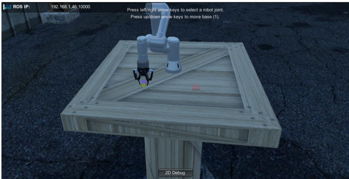
Figure 31: UR3 grabbing the cube at the start of the pick and place operation.
