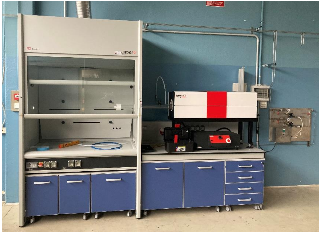
Figure 33: CVD reactor at Innovacarbon srl production site.
