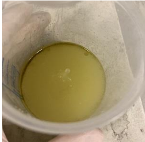
Figure 56: Acetone after regeneration of material used for adsorption of solar oil.
