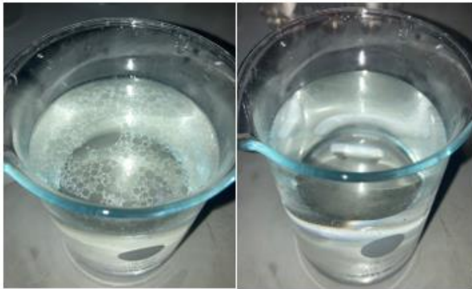
Figure 55: 12 g of Solar oil in water and treated solution with Innovacarbon material.
