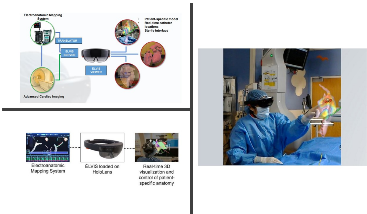
Figure 1.6: Left: Workflow for \bar{E}LVIS . From the electroanatomic mapping system, data flows to the \bar{E}LVIS application which runs on Microsoft HoloLens. Through the headset, the real-time patient-specific data is displayed in 3D. Right: holographic information provided by ELVIS .
