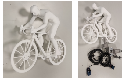
Figure 5: 3D printed model of the cyclist and model integrated with the wind tunnel setup and transducers.
