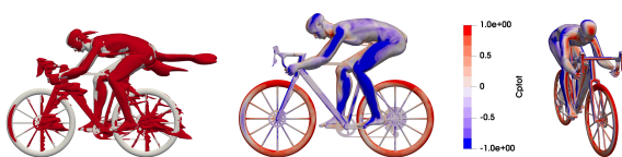
Figure 9: Total pressure coefficient on cyclist and bicycle surfaces, and isosurfaces for C_{p_{tot}} = 0
