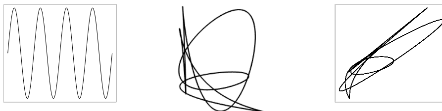
Figure 6.1: Left: \sin(t) . Center: 3-dimensional embedding with function G(x) = \sin(10x) . Right: 2-dimensional delay coordinates.
