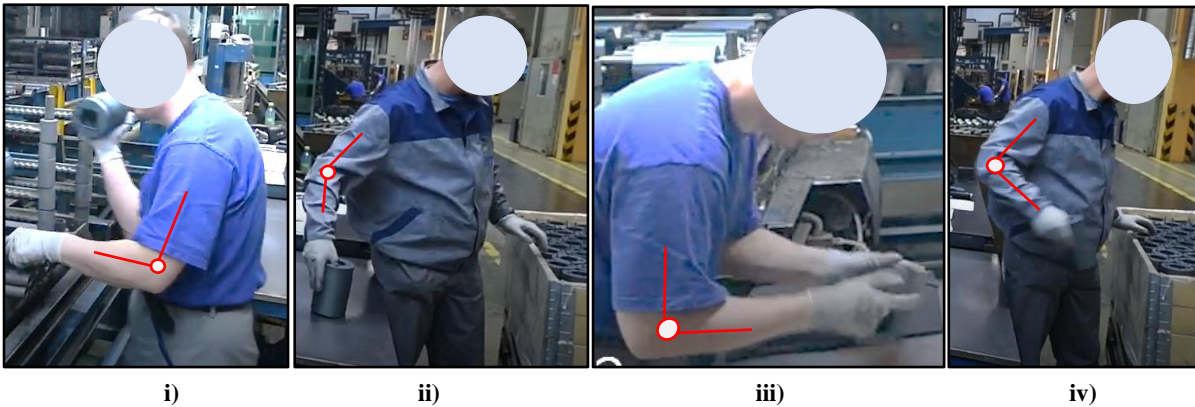
Figure 2.1: The screenshots of the industrial use-case of the European project SOPHIA. Max elbow position is \theta = 80^\circ \pm 5^\circ .
