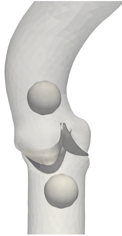
Figure 4.4: Control volumes location with respect to the leaflets.
