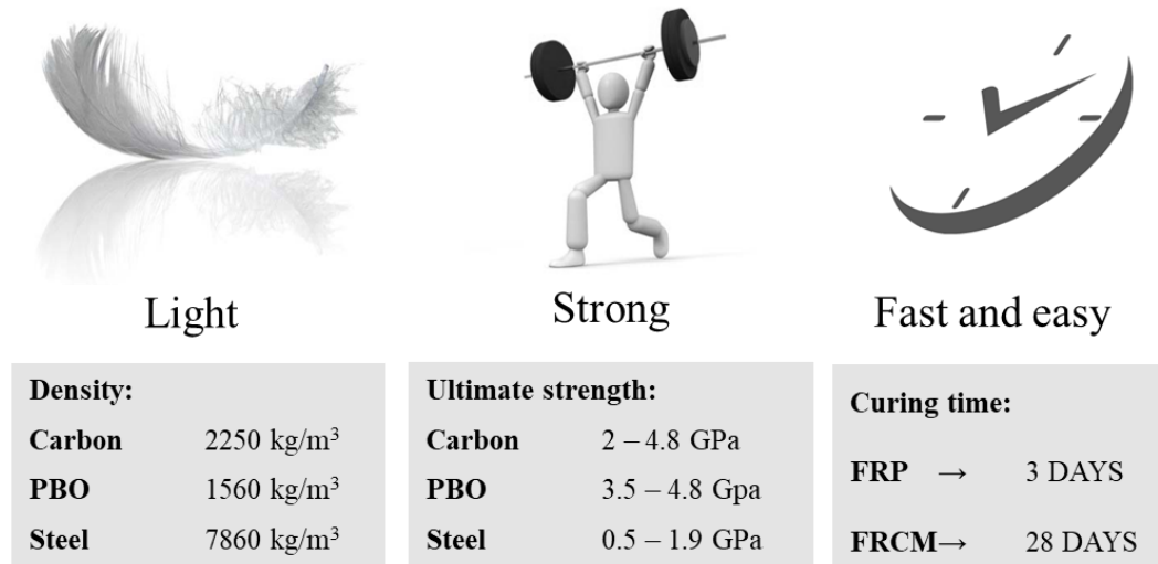
Figure 2.1: General advantages of composite materials for structural applications
