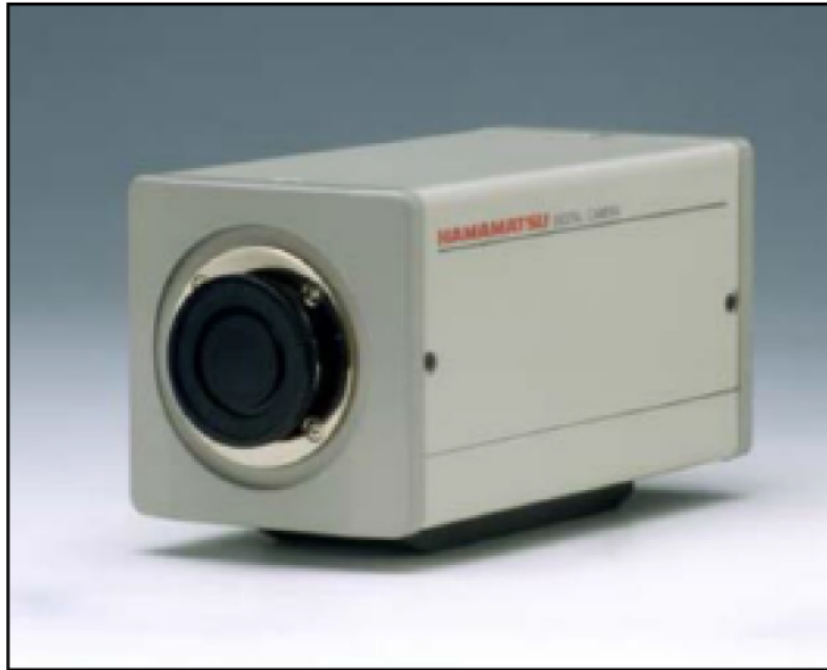
Figure 2.2: Picture of the CCD camera used for BOS image acquisitions.
