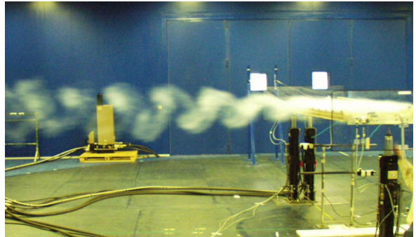
(b) Vortex shedding observed in the Bovisa wind tunnel.
