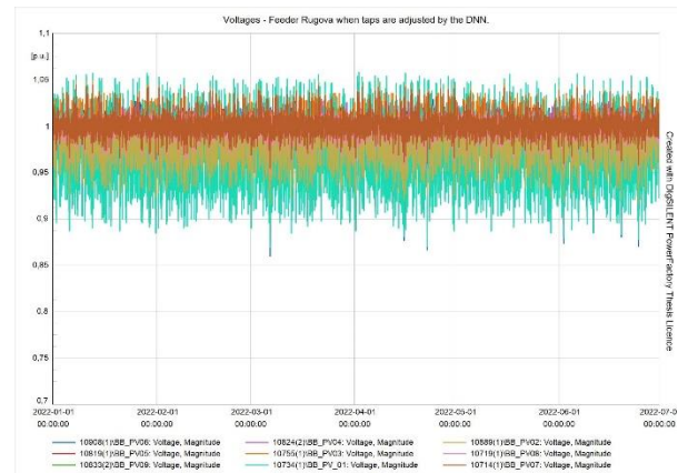
Figure 22. Feeder 2 voltages when the DNN predicts the tap positions [p.u].
