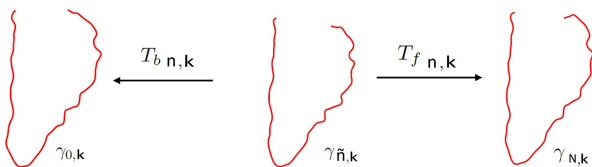
Figure 1: Scheme of application of the forward and backward transformations, respectively T_{f n,k} and T_{b n,k} , in the procedure for automatic registration (see Section 2.2) of contours \gamma_{n,k} (red lines).
