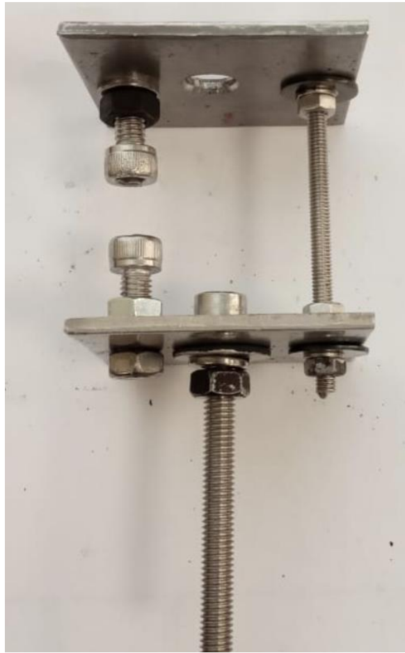
Figure 22. Sample holder to deposit Cr on corners of electroplated samples.
