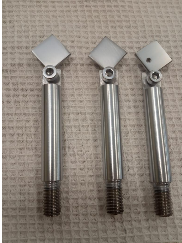
Figure 23. Sample holders for magnetron deposition onto Zr-1Nb samples.
