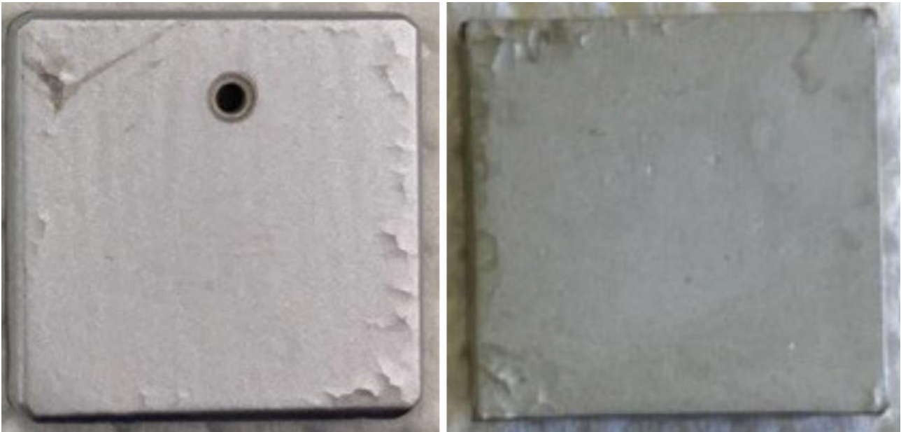
Figure 37. Effect of high current density on Zr-1Nb samples in presence of fluorides.
