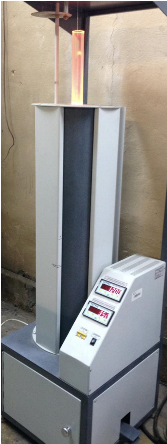
Figure 24. The ITM facility for high-temperature oxidation in steam. On the left it is in operation, on the right its scheme (1. Quartz reaction tube; 2. Tube furnace; 3. Specimen location; 4. Pt/Rh-Pt Thermocouple; 5. Control unit; 6. Drip evaporator; 7. Water tank; 8. Heater).
