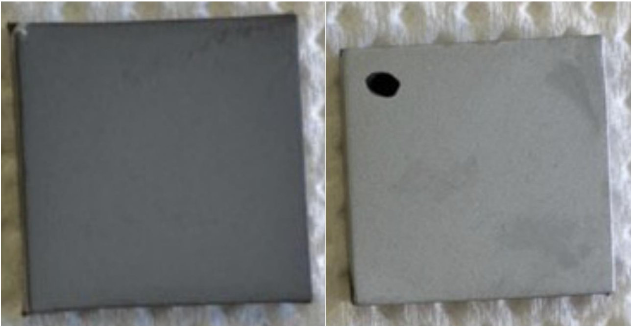
Figure 41. Cold chromium plated sample on the left (35 \mu\text{m} thick), and chromium plated following the procedure described below on the right (18 \mu\text{m} thick). Both the deposition processes lasted 75 minutes on Zr-Nb samples.
