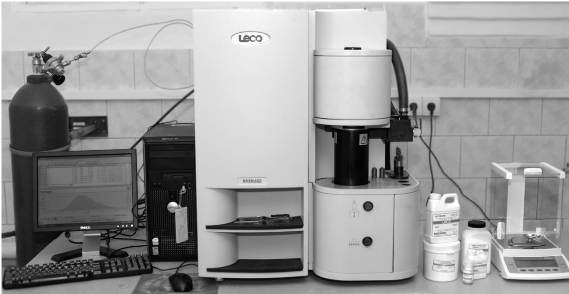
Figure 28. LECO installation for hydrogen content measuring in metals or alloys.
