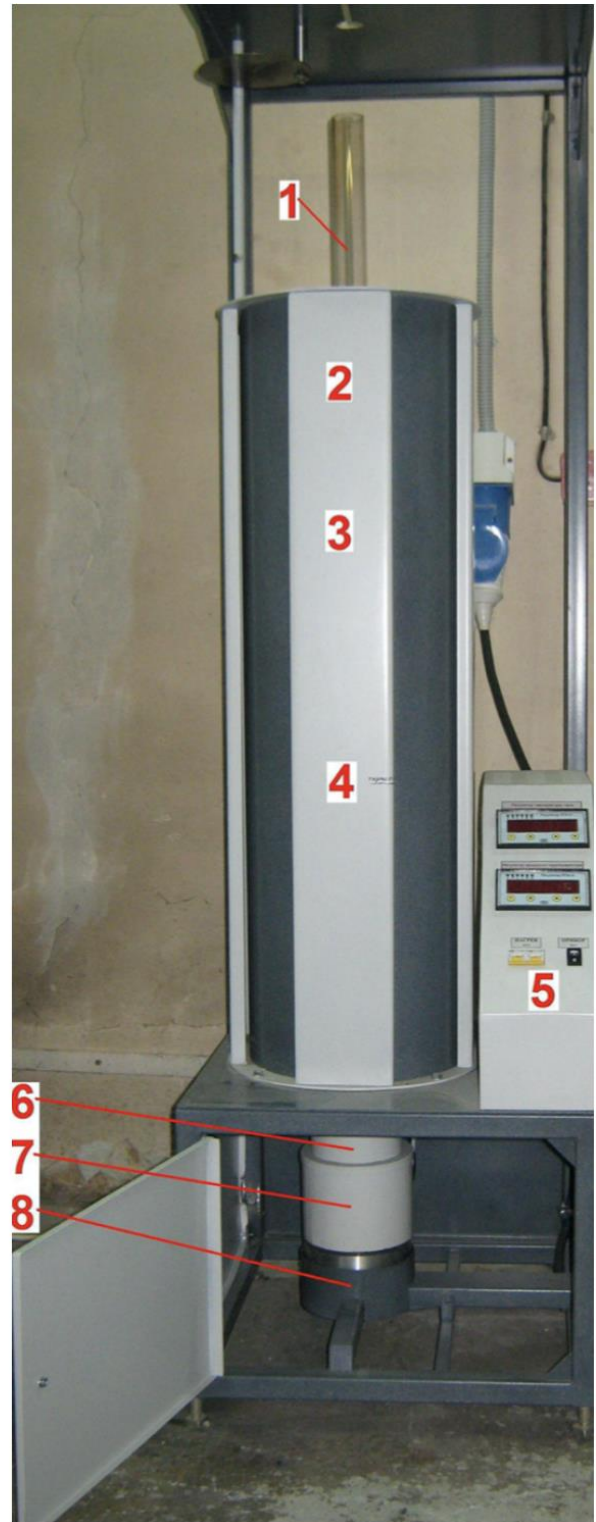
Figure 24. The ITM facility for high-temperature oxidation in steam. On the left it is in operation, on the right its scheme (1. Quartz reaction tube; 2. Tube furnace; 3. Specimen location; 4. Pt/Rh-Pt Thermocouple; 5. Control unit; 6. Drip evaporator; 7. Water tank; 8. Heater).
