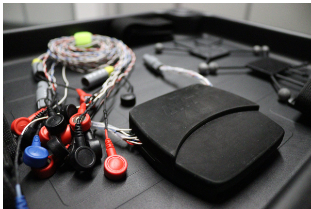
Figure 9: Data acquisition platform: 8-channels sEMG wearable sensor board. Two sides, four channels for each side.
