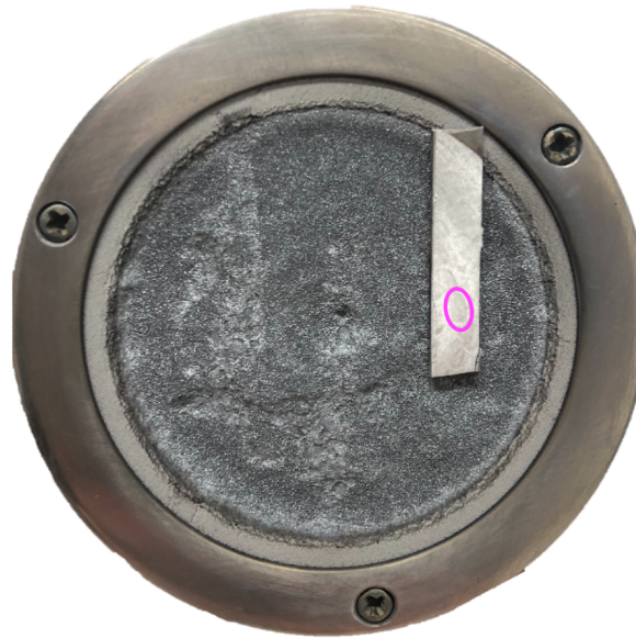
Figure 5.11: Photograph of the boron target with a tungsten piece employed for the production of B/W films. One of the laser spot traces is circled in pink.
