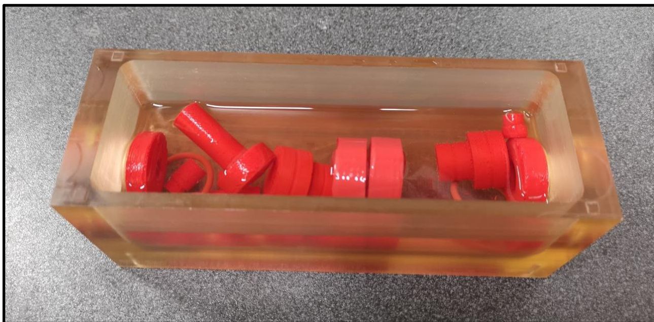
Figure 3.4 The 3D printed components were left in a 70% EtOH bath inside the chamber for 5 hours to provide sterility.
