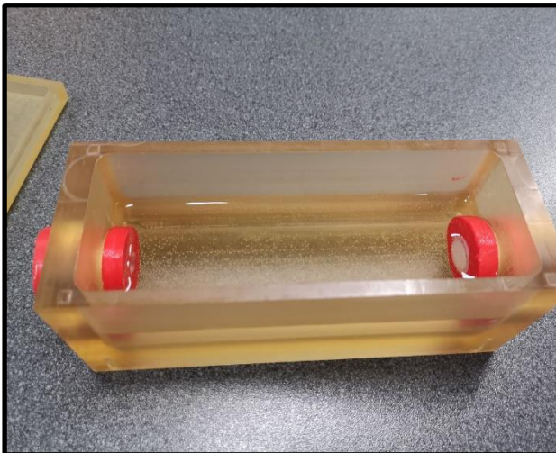
Figure 3.7 The sterilized PBS-filled bioreactor showed no sign of contamination after one day of culture in incubator.
