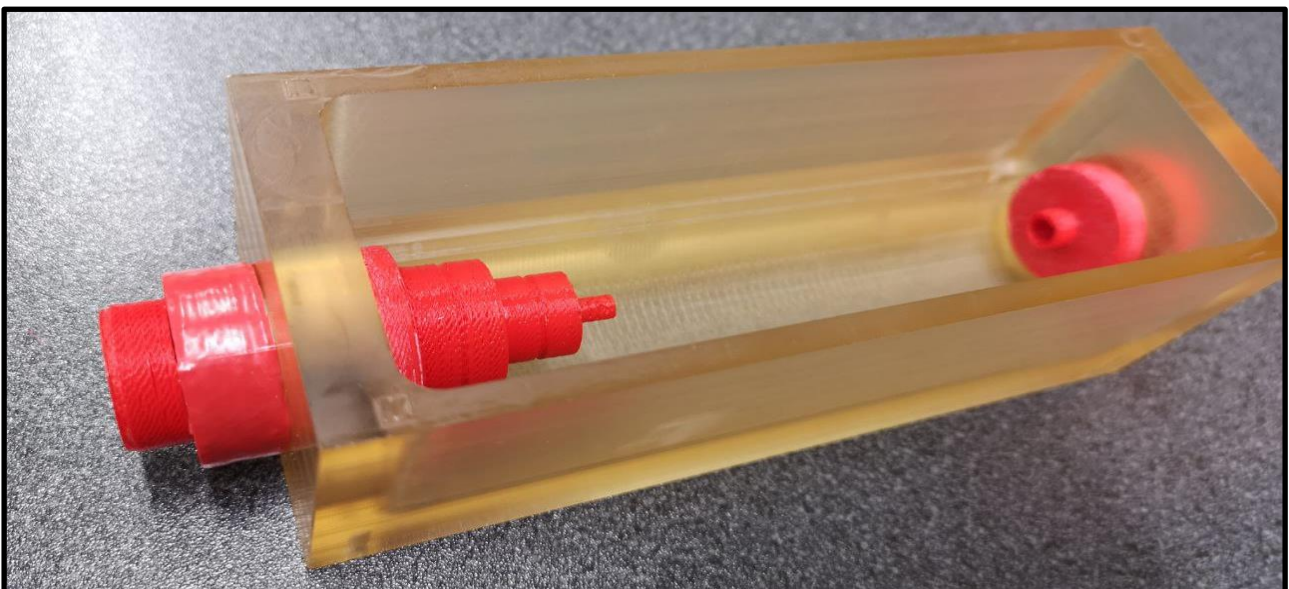
Figure 4.2 The fully assembled bioreactor from different perspectives. It is possible to appreciate the two inlets fully assembled along with the fixed grip. It was not possible to place the mobile grip due to the absence of the perfusion axis.
