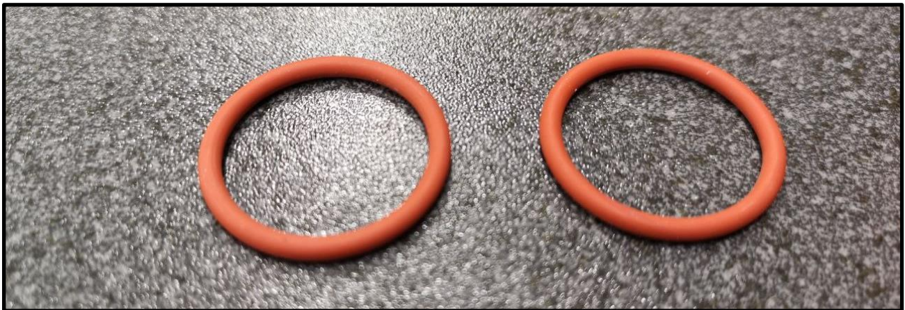
Figure 4.4 The O-rings used to enhance the sterility maintenance and the water seal were too thick to be fully compatible with the etches on the 3D printed rings components.
