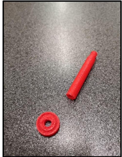
Figure 4.3 Rupture of the components often happen on the plane of linkage between volumes of different width.
