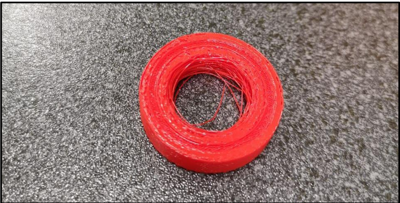
Figure 2.30 For the ring components, presenting an internal thread, it was necessary to print the inner walls before the outer ones to avoid large overhangs.
