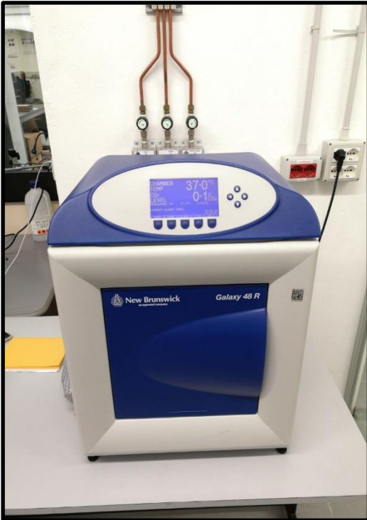
Figure 3.6 The incubator used for the sterility maintenance experiment (left). Note the values of temperature, relative humidity and CO 2 partial pressure. The sterilized PBS-filled bioreactor inside the incubator (right).
