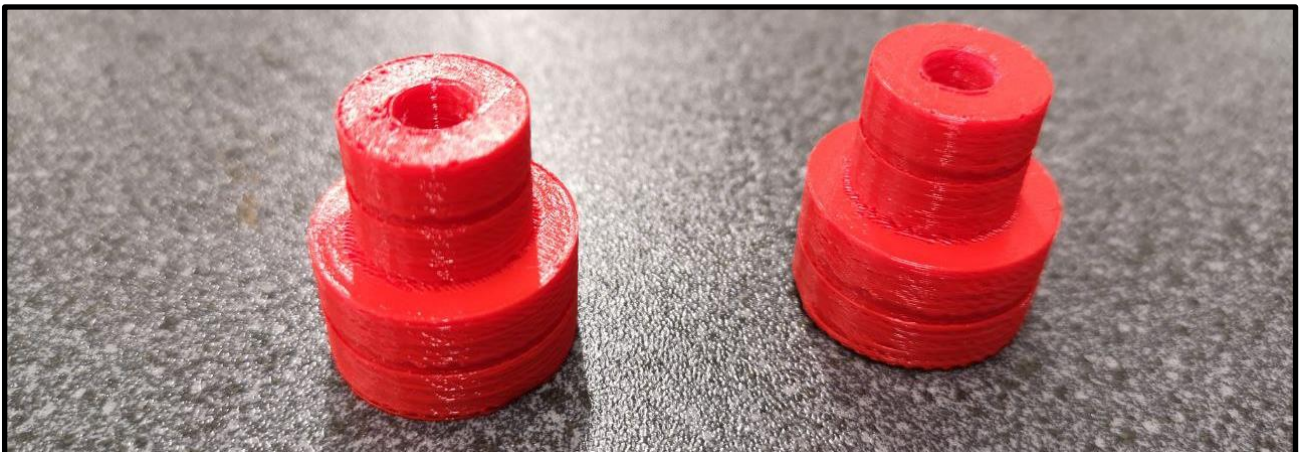
Figure 2.20 The two 3D printed scaffold grips.
