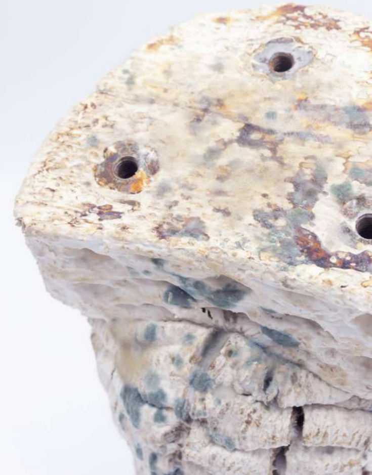
^ Img.208, 209 ^ Combined structure of clay and sawdust semicylinders 1-2, bio-welded. Detail of the threaded metal inserts into the clay matrix.
