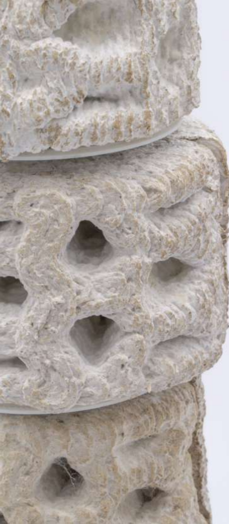
^ Img.216, 217 ^ Clay and sawdust semicylinders sample 3.
