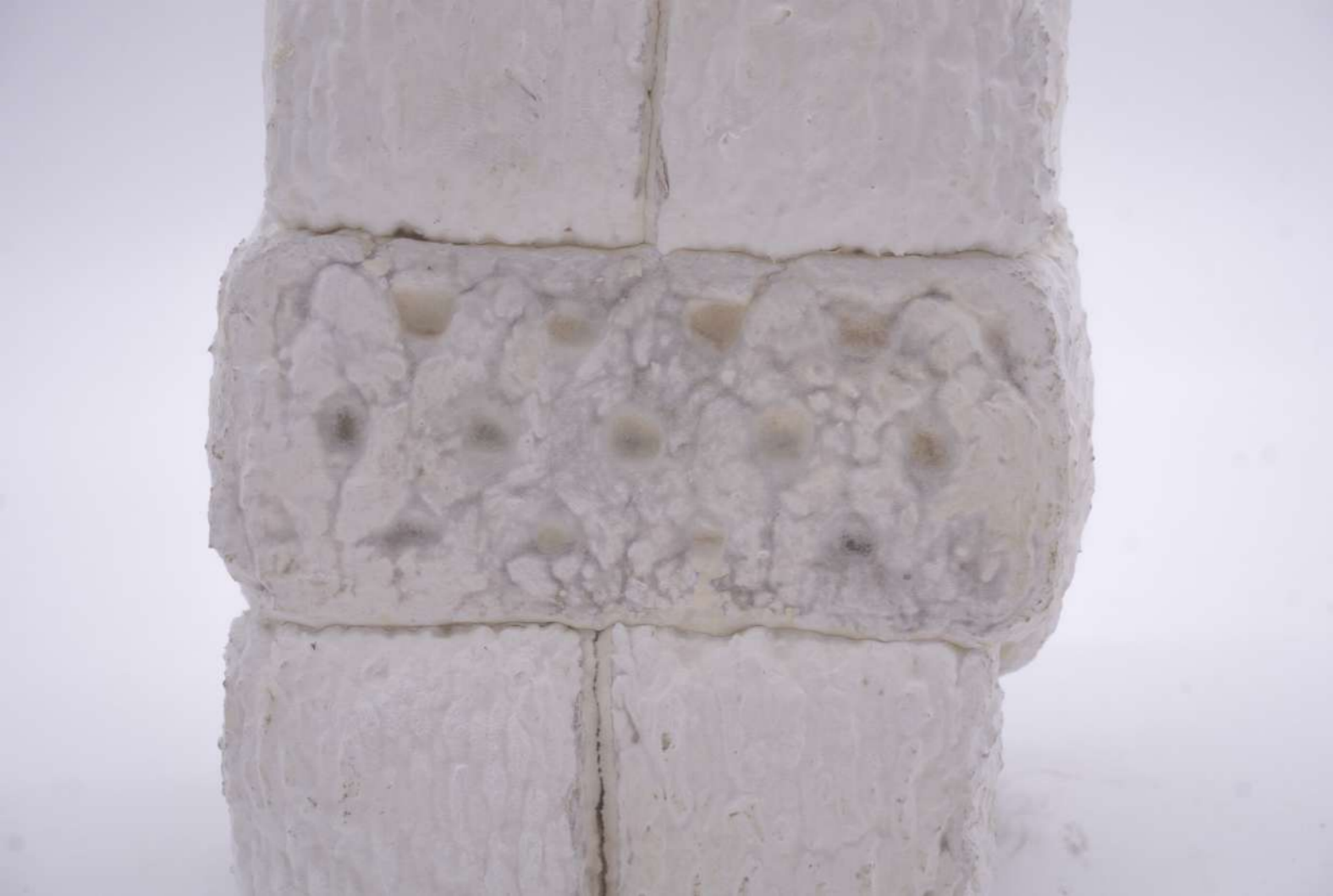
^ Img.197 ^ Detail of the bio-welding process between modules through the designing of flat surfaces to increase the contact area. This solution was found to be most useful for ensuring correct adhesion between the pieces by exploiting the weight of the material that kept the surfaces in contact during the growth process of the binding matrix.
