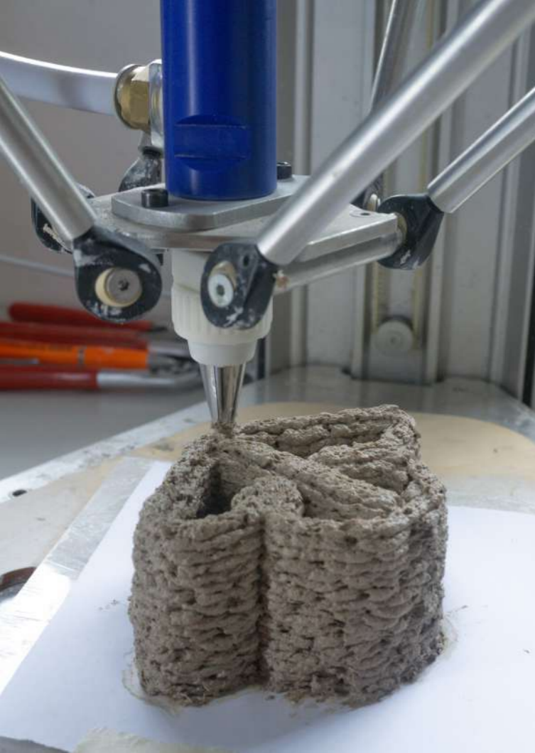
^ Img.188, 189, 190 ^ 3D printing process of the specimens through the use of the custom nozzle, which enabled blockage-free extrusion of the mixture containing a substrate larger than 1.5mm. The large size difference between the clay sediment and sawdust particles resulted in a loss of layer definition and a tendency for the material to tear during deposition. The implementation of xanthan gum was a key component in achieving better extrudability of the mixture and a partial increase in print definition.
