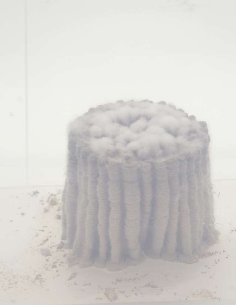
^ Img.169 ^ Inoculation by filling of the sample with the self-produced hemp substrate, progressive spreading of the mycelium on the clay matrix.
