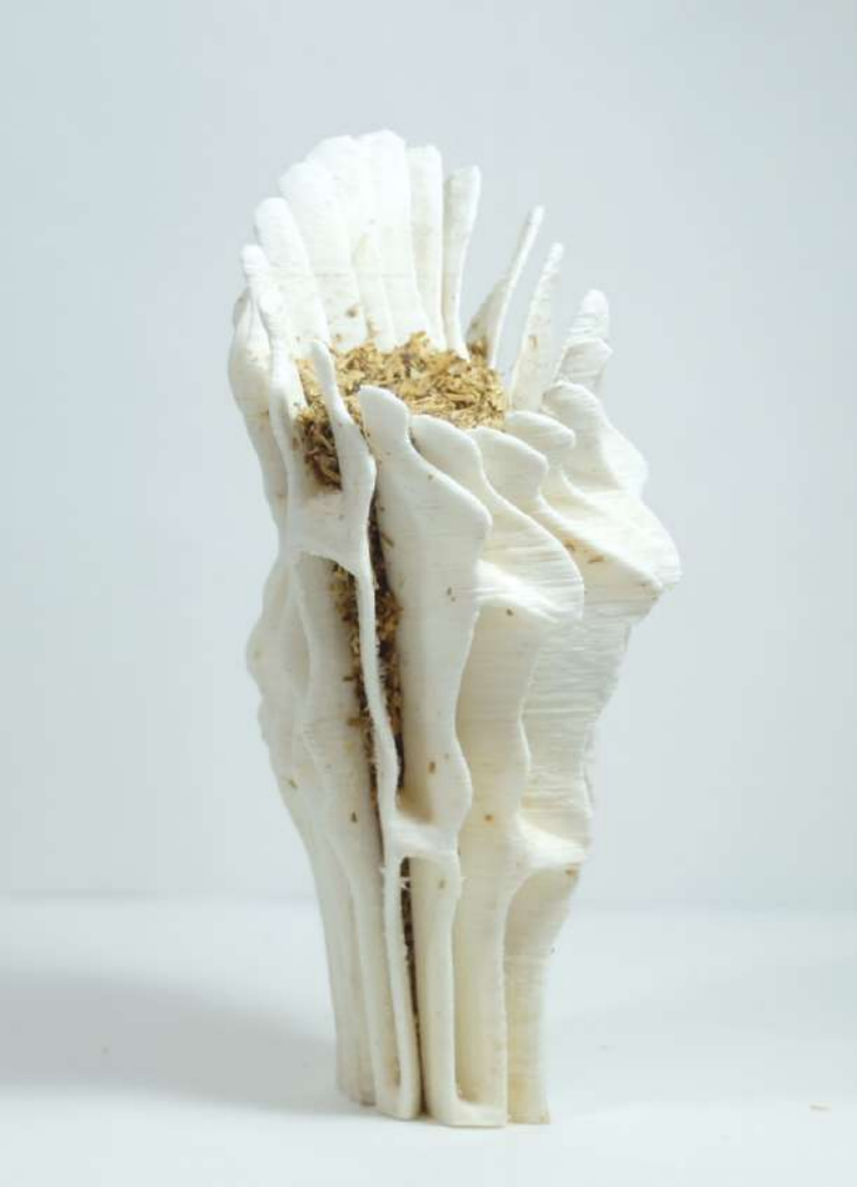
^ Img.89, 90, 91 3D printed shape investigation from the Hyper Articulated Myco Morphs project by Jessica Dias. The geometries have been computationally designed on Grasshopper to simulate the complexity of organic patterns of growth and create inlets and cavities to promote the development of the organism. The fungus, by growing between the hollows parts creates a dense matrix which acts as a solid reinforcement.
