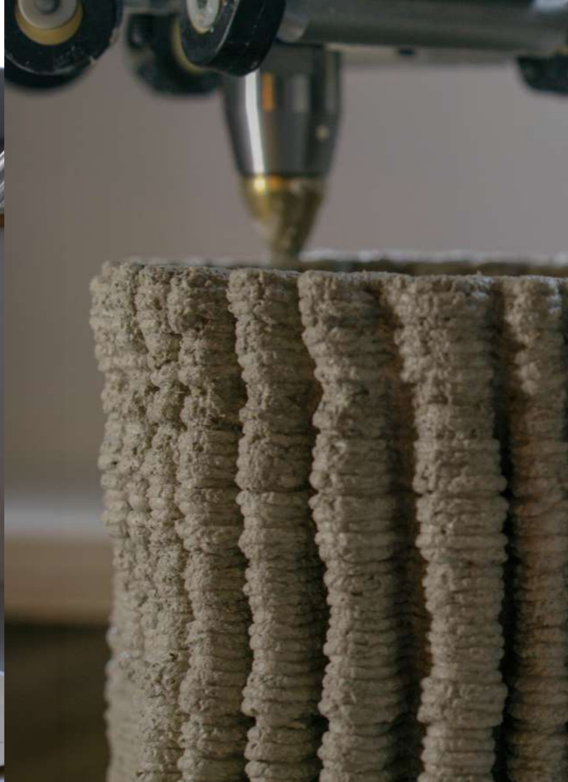
^ Img.173, 174, 175 3d printing process of Parametric growth clay and hemp samples 1-2. The intricacy and the corrugation of the geometries were parametrically designed to enhance stability during printing and to favor the organism's growth through the creation of humidity niches and the proximity of walls to be filled by the fungal matrix.
