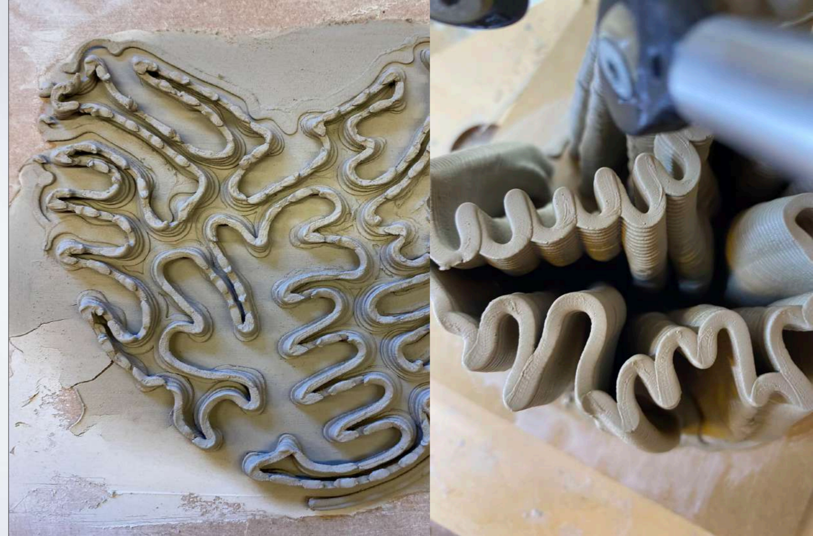
^ Img.161, 162 ^ Details of the sample's bottom and top printing paths generated through parametric modelling on Grasshopper.
