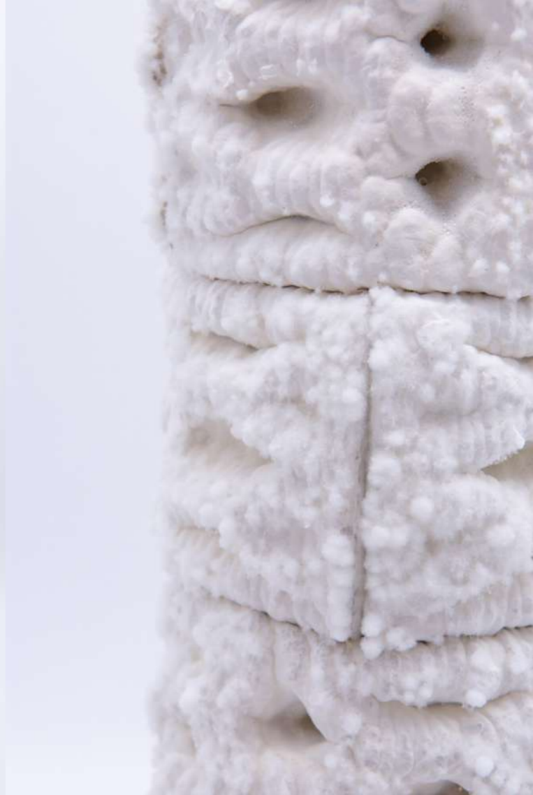
^ Img.237, 238, 239 ^ Close-up and on-framework views of the assembled leg at the end of the second growth cycle. The extended growth period played a crucial role in restarting the organism's growth and enabling the bio-welding process to occur between the individual modules and levels.
