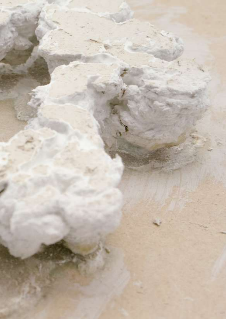
^ Img.180 ^ Details of parametric growth clay and sawdust sample 1 showing no growth of organisms on the piece's bottom surface and yellow stains on the upper layers due to contamination occurred during drying. Difficult removal of the piece from the MDF base due to excessive drying.
