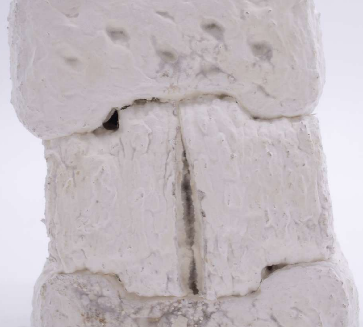
^ Img.196 ^ Detail of the bio-welding process between modules through the designing of connection features to increase contact surfaces on multiple directions. This solution resulted inconsistent due to the difficulties encountered to obtain precise geometry with the material mixture.
