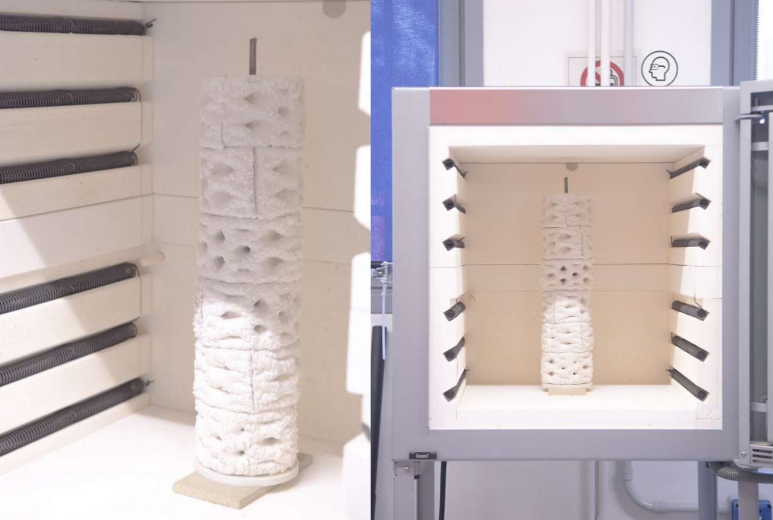
^ Img.240, 241 ^ Views of the assembled artifact removed from the support framework and ready to undergo the thermal deactivation process.
