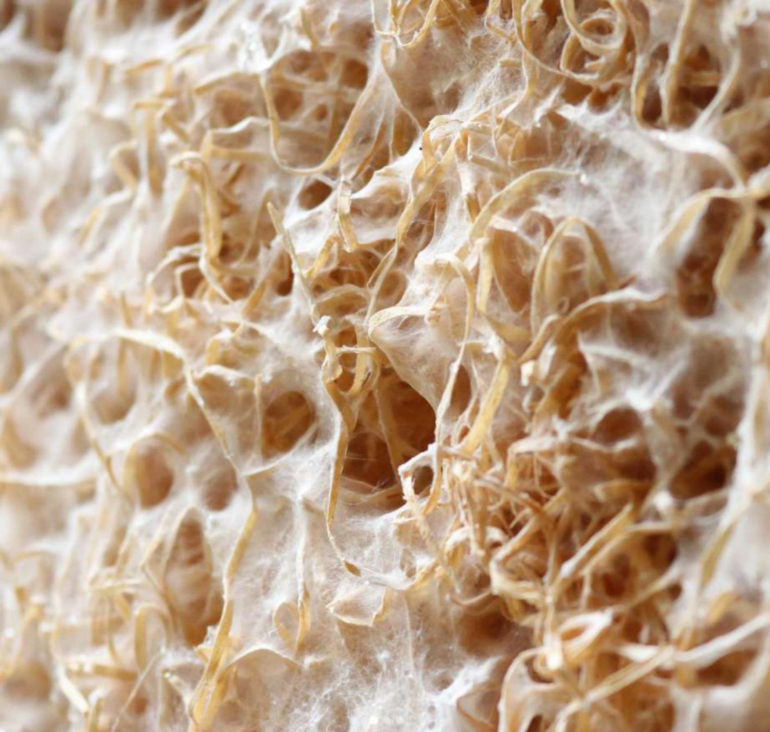
^ Img.59 Actively collaborating with the living material throughout the design and production of the sound absorbing panel, a flexible room divider is formed within a pre-designed mould as the mycelium grows over and bonds with a mixture of plant fibers. Close-up view of the filaments spreading on the substrate’s particles, from Jonas Edvard’s acoustic wall “MYX Sail / Floor” made in mycelium and plant fibers showcased at “The Mindcraft Project 2023”.
