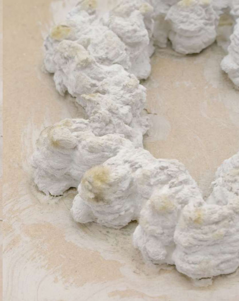
^ Img.180 ^ Details of parametric growth clay and sawdust sample 1 showing no growth of organisms on the piece's bottom surface and yellow stains on the upper layers due to contamination occurred during drying. Difficult removal of the piece from the MDF base due to excessive drying.
