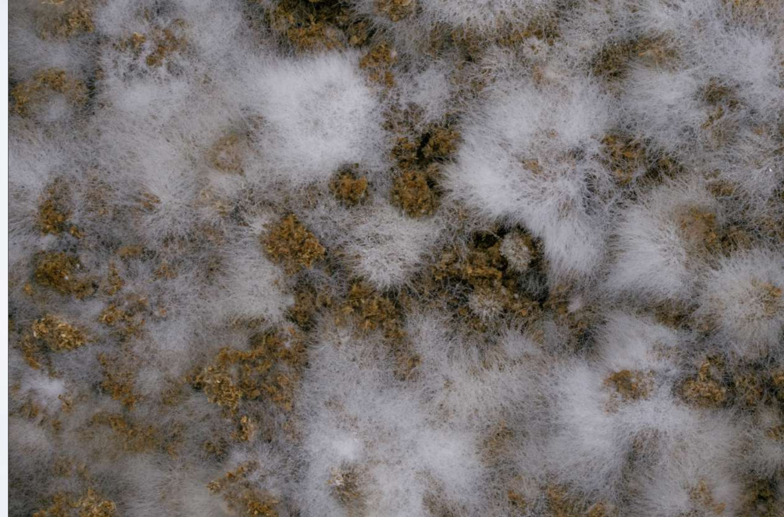
^ Img.126 ^ Close-up of substrate contamination with the outbreak of external organisms on the hemp occurred after the inoculation strategy performed by blending and dispersing the selfproduced grain spawn.
