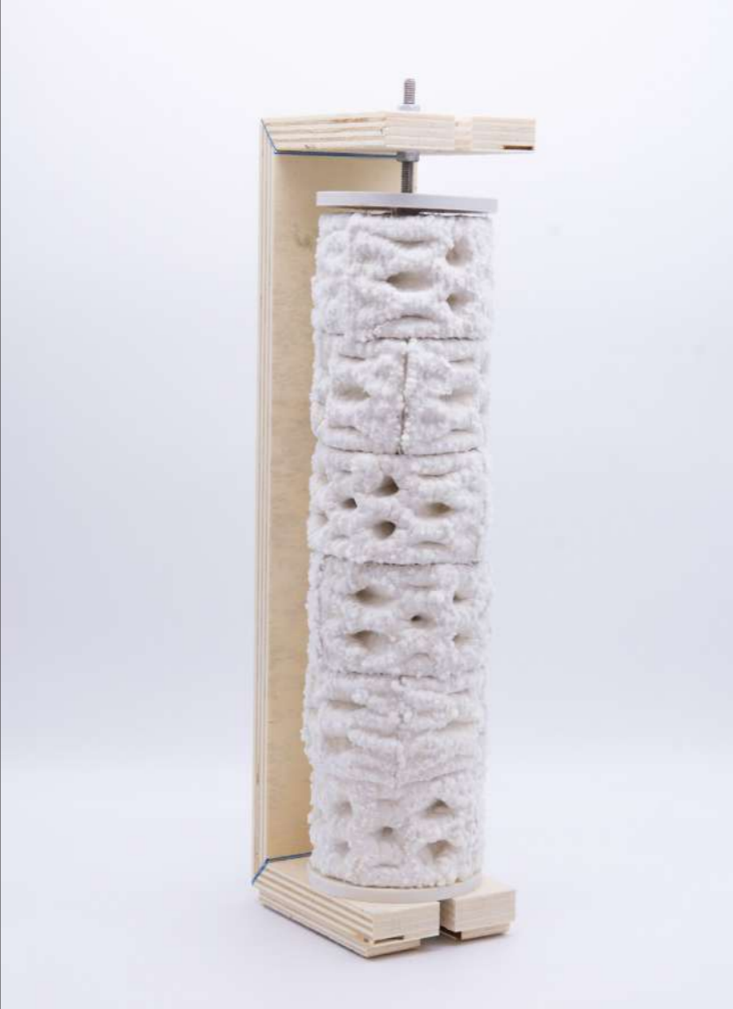
^ Img.237, 238, 239 ^ Close-up and on-framework views of the assembled leg at the end of the second growth cycle. The extended growth period played a crucial role in restarting the organism's growth and enabling the bio-welding process to occur between the individual modules and levels.
