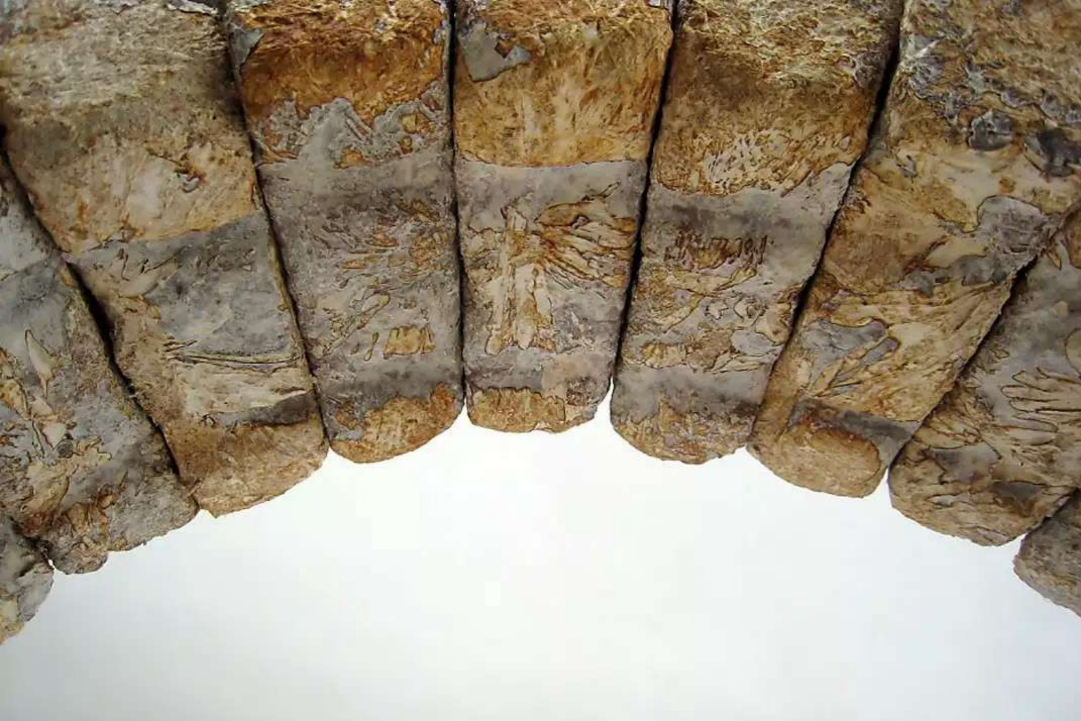
^ Img.75, 76 ^ Mycelium arc and sculptures built by using bricks made of MBC, Philip Ross. By using mycelium bricks, the artist has created artifacts that showcase both the structural capabilities and the aesthetic appeal of this organic material. Through his work, Philip Ross encourages a reevaluation of traditional construction methods and promotes the integration of innovative and environmentally friendly solutions into contemporary design and sculpture.
