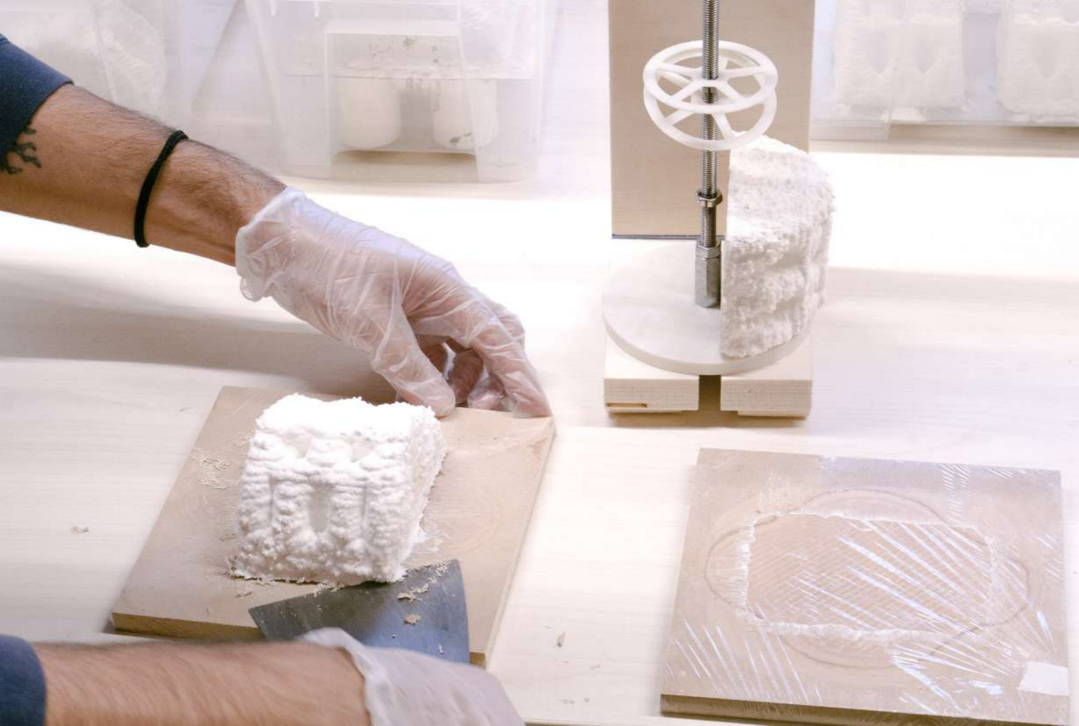
^ Img.232, 233, 234 ^ Stacking the modules during fabrication of one of the Terraforma legs. The assembly phase was carried out using the specific framework designed to control the weight distribution of the pieces and prevent deformations.
