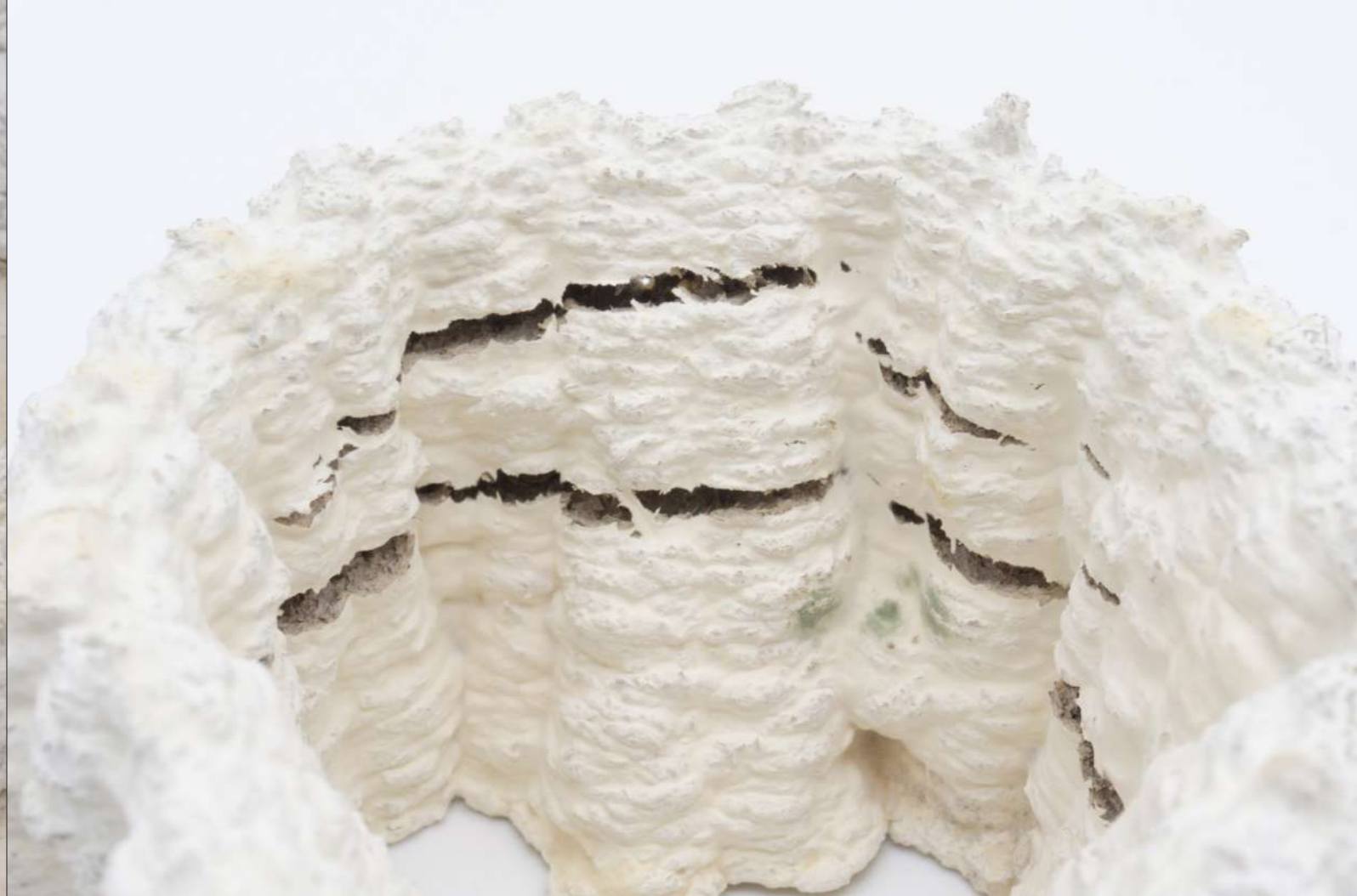
^ Img.181 ^ Close-up view of the cracking occurred on the parametric growth clay and sawdust sample 2 after deactivation and due to excessive residual moisture and thermal shock.
