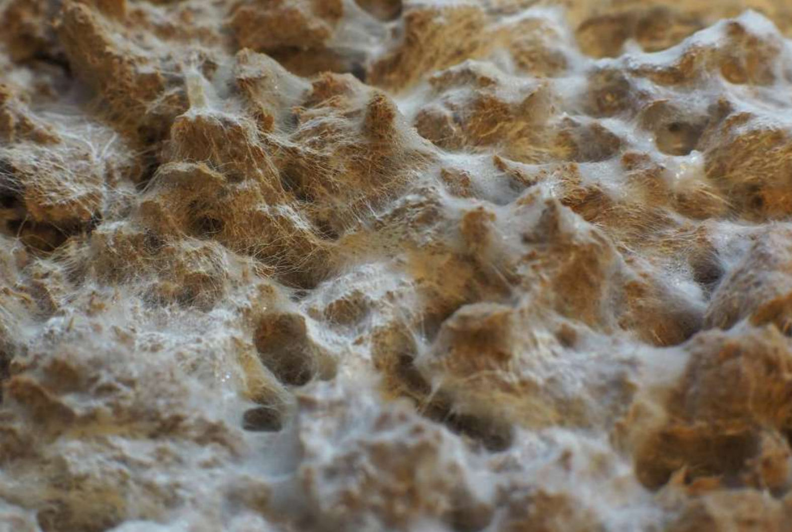
^ Img,93,94 On the left page close-up view of the colonised material surface of the Protomicokion column, on the right one detailed view of the intricate geometry of the modules, designed to improve the stiffness of the structure in order to make it a self-standing architectural element.
