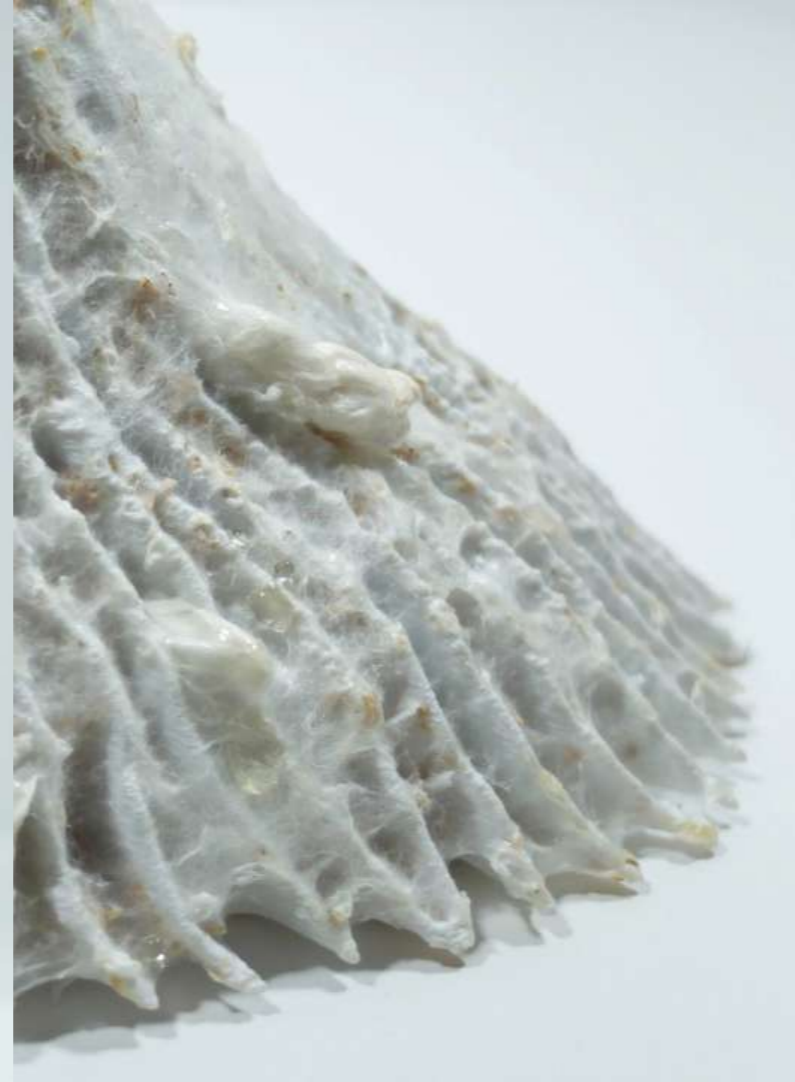
^ Img.89, 90, 91 3D printed shape investigation from the Hyper Articulated Myco Morphs project by Jessica Dias. The geometries have been computationally designed on Grasshopper to simulate the complexity of organic patterns of growth and create inlets and cavities to promote the development of the organism. The fungus, by growing between the hollows parts creates a dense matrix which acts as a solid reinforcement.
