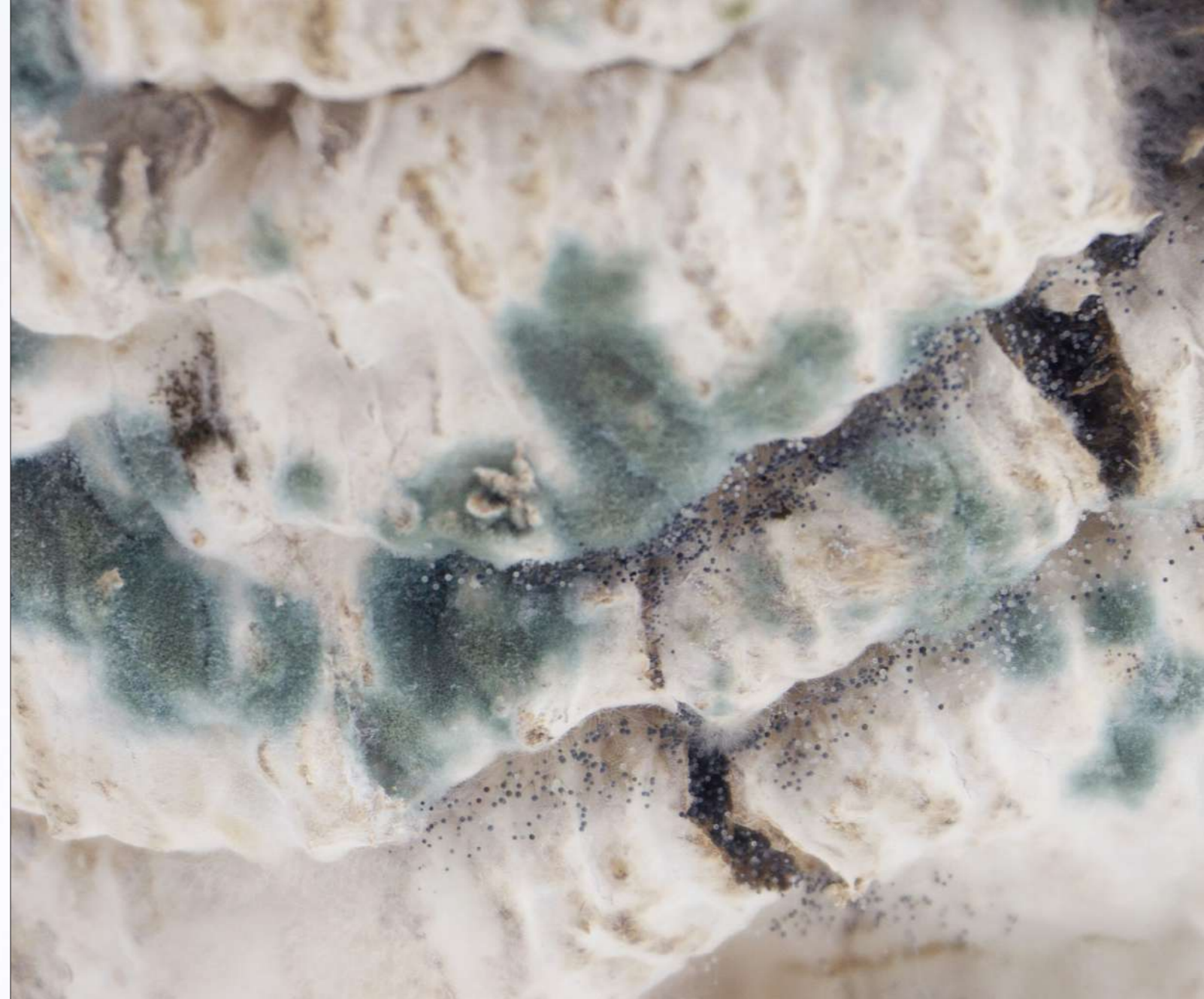
^ Img.210, 211 ^ Detail of contamination on the combined structure of clay and sawdust semicylinders 1-2. Growth of several kind of organism was observed on the surfaces due to insufficient drying and handling of the pieces which led to the outbreak of green-blue mold and black dots.
