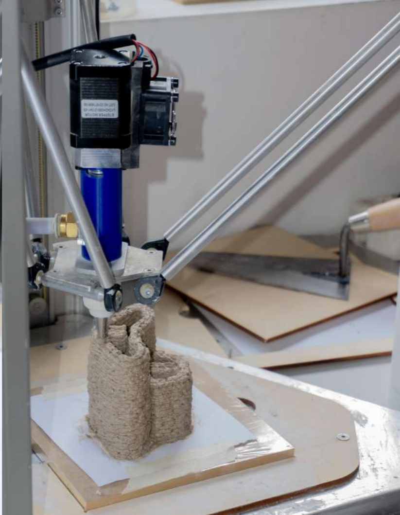
^ Img.188, 189, 190 ^ 3D printing process of the specimens through the use of the custom nozzle, which enabled blockage-free extrusion of the mixture containing a substrate larger than 1.5mm. The large size difference between the clay sediment and sawdust particles resulted in a loss of layer definition and a tendency for the material to tear during deposition. The implementation of xanthan gum was a key component in achieving better extrudability of the mixture and a partial increase in print definition.
