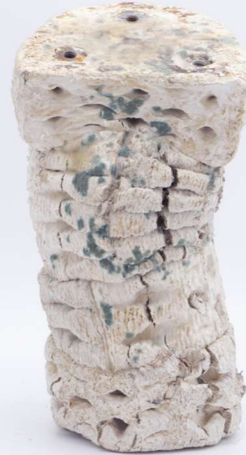
^ Img.208, 209 ^ Combined structure of clay and sawdust semicylinders 1-2, bio-welded. Detail of the threaded metal inserts into the clay matrix.
