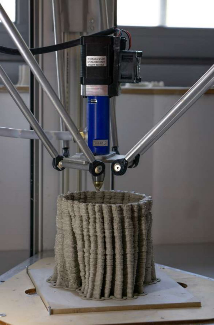
^ Img.173, 174, 175 3d printing process of Parametric growth clay and hemp samples 1-2. The intricacy and the corrugation of the geometries were parametrically designed to enhance stability during printing and to favor the organism's growth through the creation of humidity niches and the proximity of walls to be filled by the fungal matrix.
