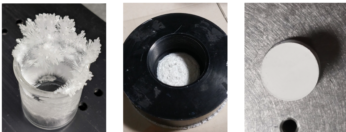
Figure 3.18: From left to right: NaDPA crystals, once its solution is completely evaporated; drying stage for NaDPA paste disk in its housing; finished NaDPA disk.
