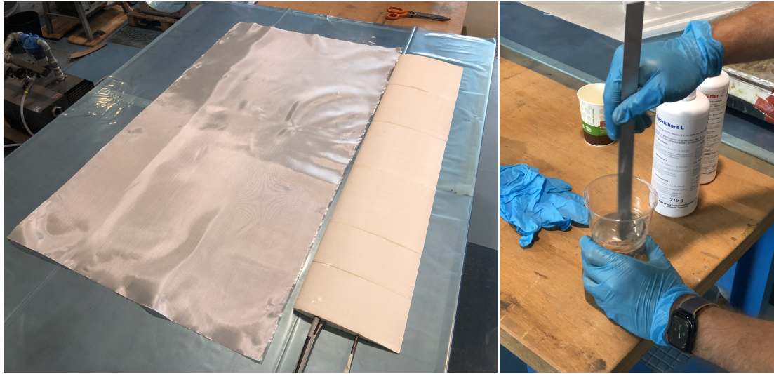
(a) Glass-fiber cloth and foam wing
