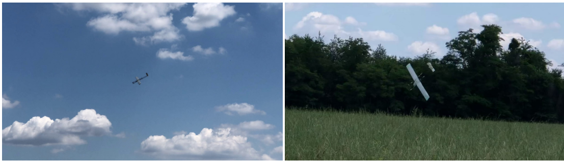
Figure 2.12: June 12th crash final moments; significant torsion can be observed at the wingtip.
