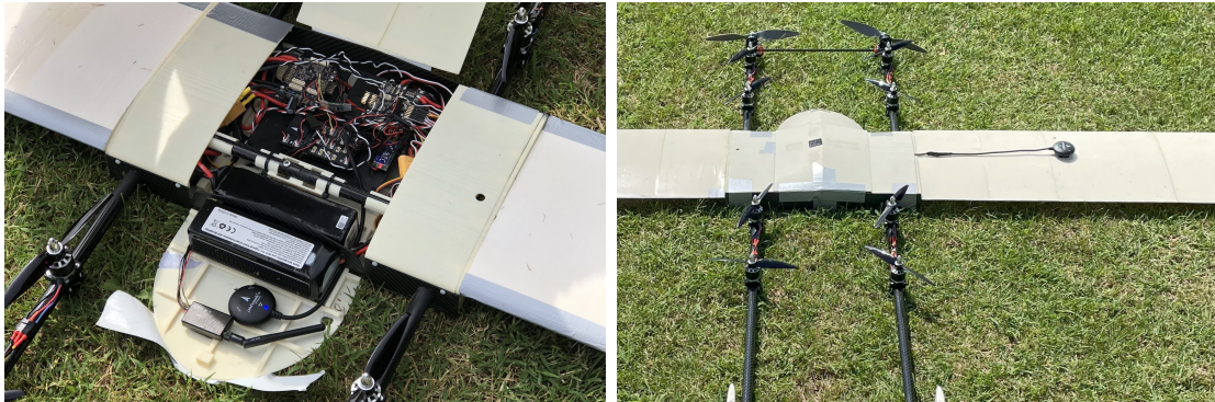
(a) Original GPS module positioning inside the fuselage (b) GPS module positioning on the right wing fuselage
