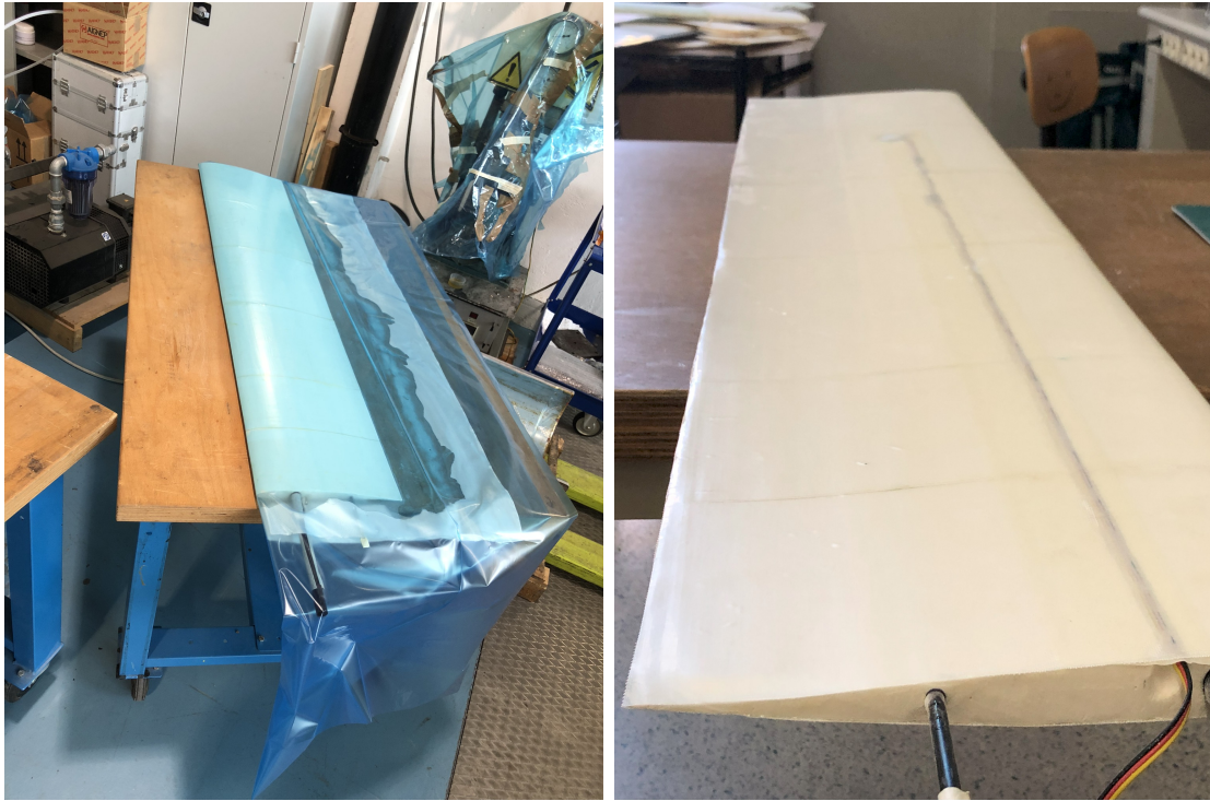
(a) Cladded wing during curing phase
