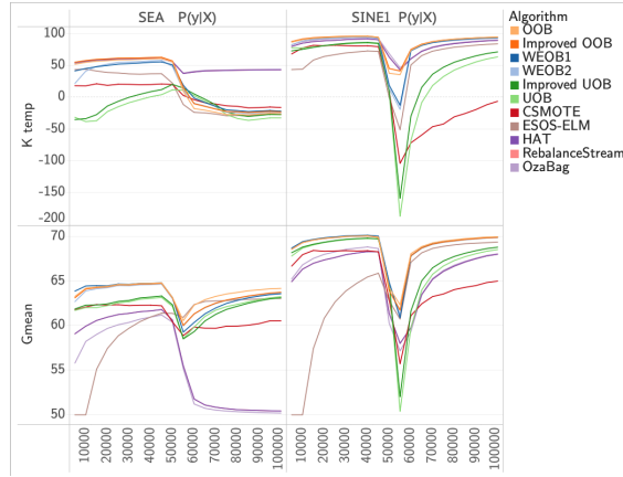
Fig. 5: K_{temp} and Gmean during SEA and SINE1 streams having a P(y|X) drift and imbalance ratio 1:9
