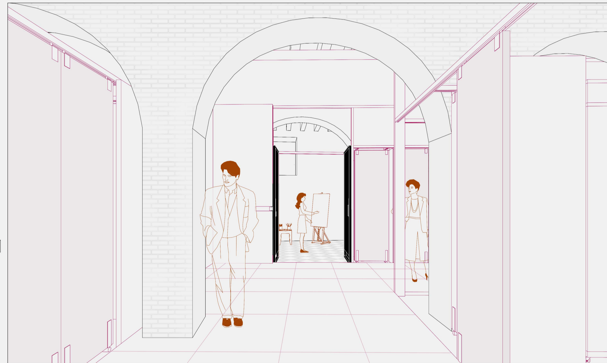
Movable Partitions Type 2 --- Rotating Doors: To close or open the entrance of each studio
