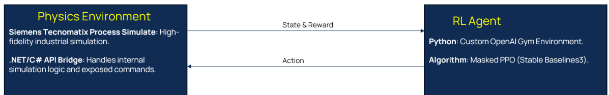
Figure 5.2: Architecture of the communication bridge: The Python script (Agent) communicates with the C# Simulation Controller via TCP/IP.
