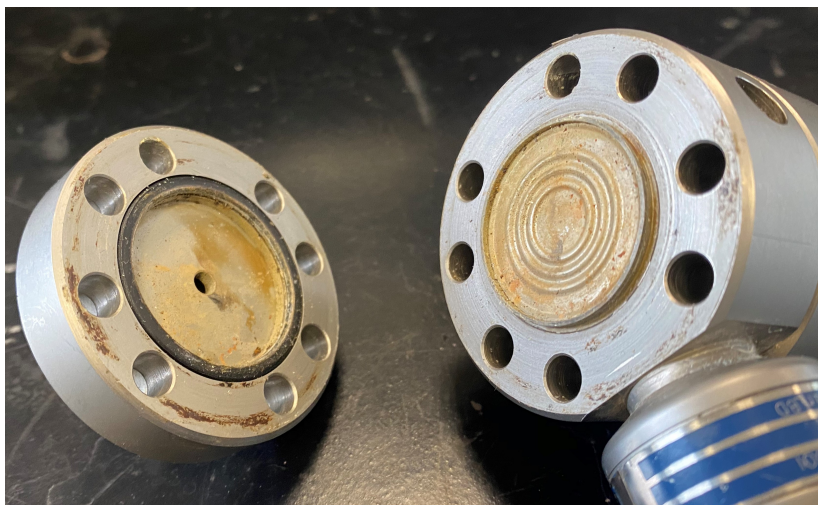
Figure 7.9. Internal membrane chamber of a Schaevitz differential pressure transducer.
