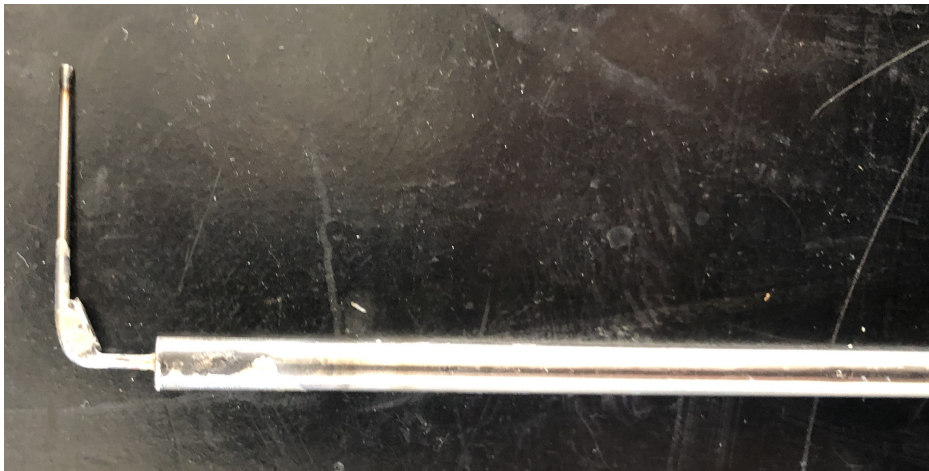
Figure 3.19. TotAle simple Pitot tube.
