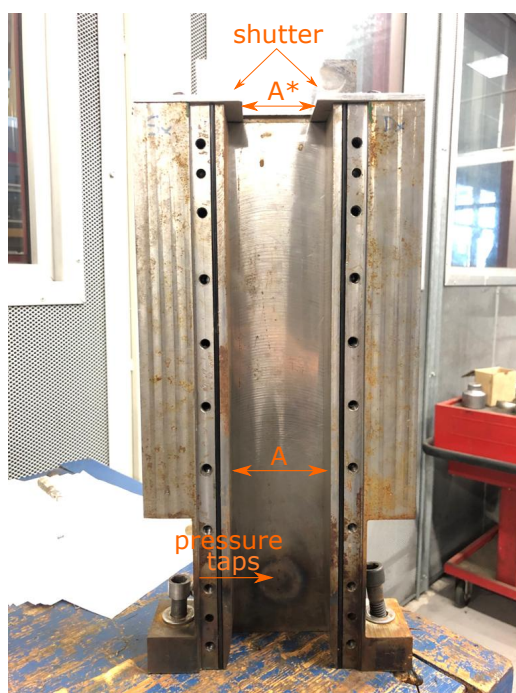
Figure 7.1. Choked convergent nozzle employed in the experimental campaign at the Safety Valves Test Rig .
