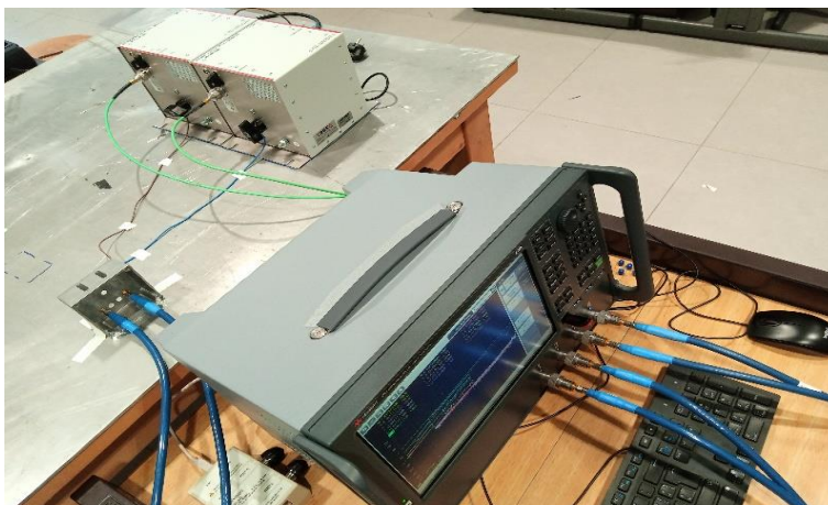
Figure 5.10: Experimental test bench to characterize the LISN.
