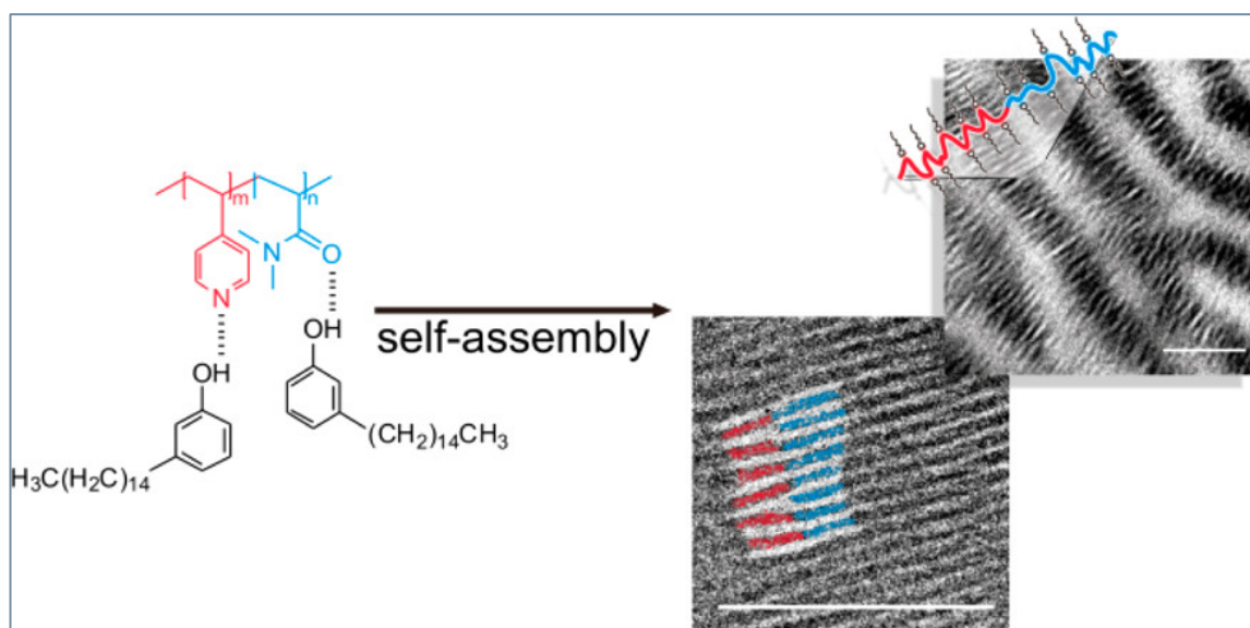
Figure 1.5: Schematic representation and TEM images of the P4VP-b-PDMA(PDP) supramolecular complex. [46]
