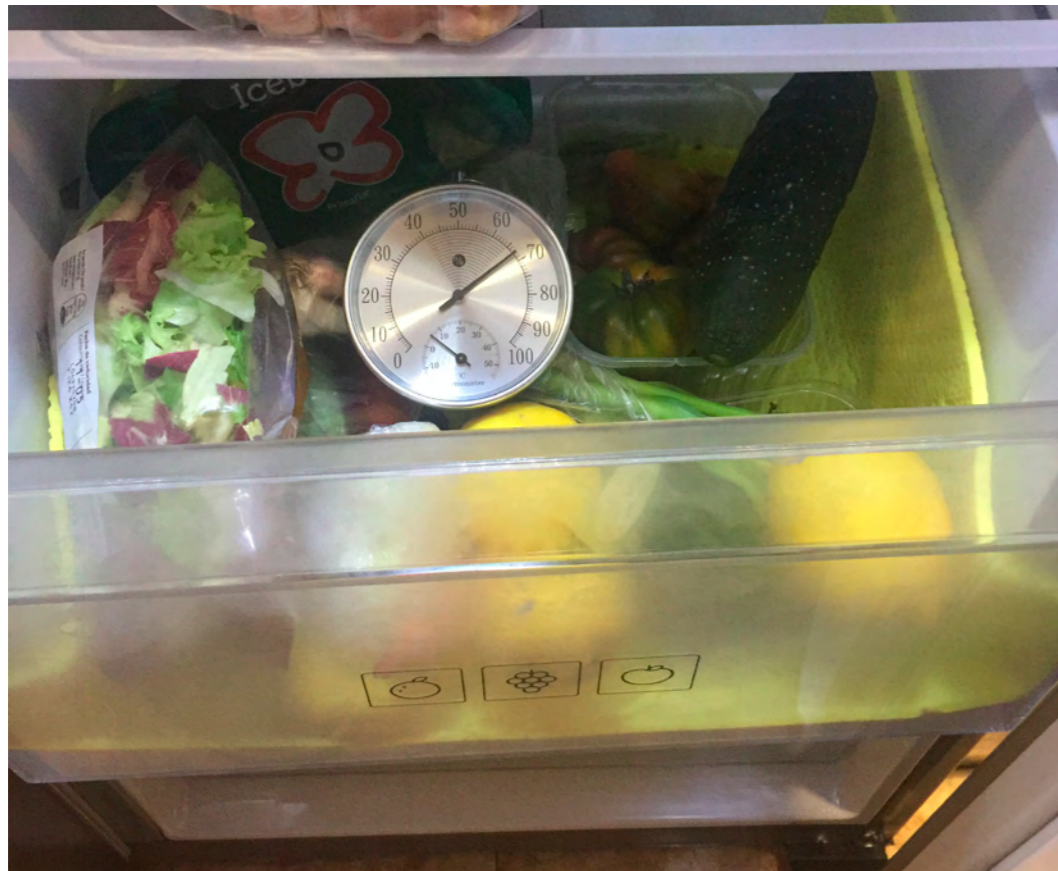
Fig.87 Upper 'crisper drawer' of Samsung refrigerator provides conditions of 70% RH and temperature of 5°C.
