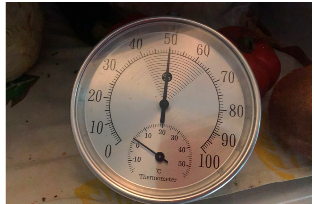
Fig.92 Measuring RH and temperature inside the 'crisper drawer' of Bosch Refrigerator Series 2.
