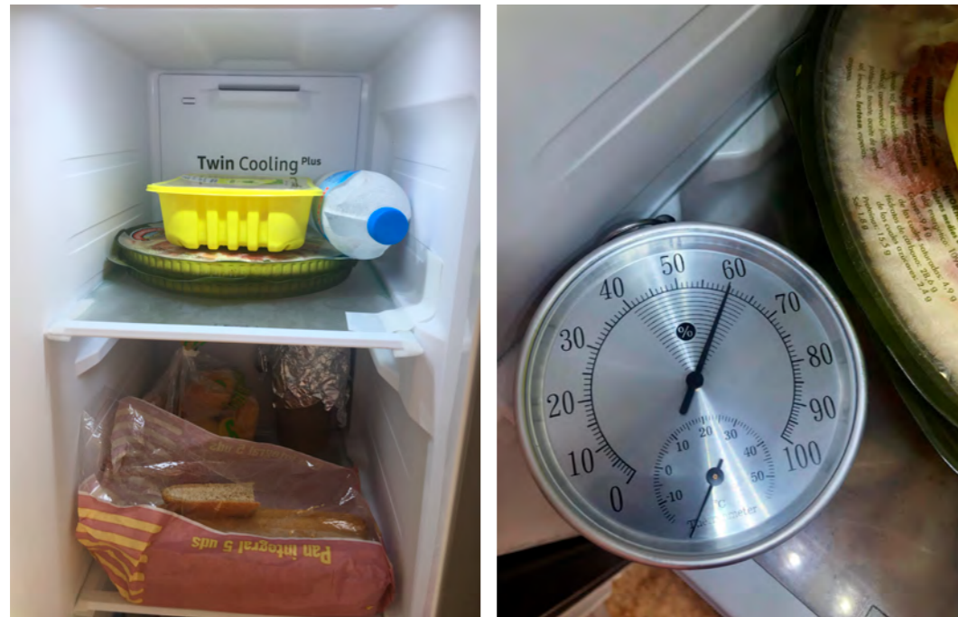
Fig.84 The left side of Samsung refrigerator (freezer side) uses conditions of 60% RH and temperature around -19^{\circ}\text{C} .
