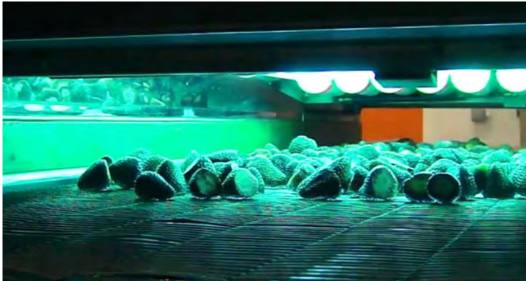
Fig. 143 UV-C light tunnel used for industrial food sanitizing. Source: Youtube.
