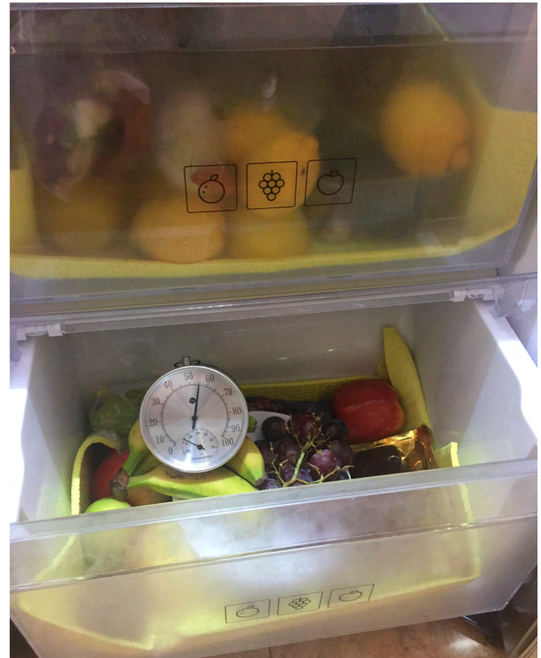
Fig.88 Lower 'crisper drawer' of Samsung refrigerator provides conditions of 55% RH and temperature of 5°C.
