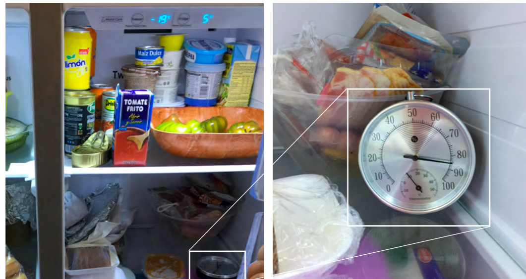
Fig.85 The right side of Samsung refrigerator, uses conditions of 85% RH and temperature around 10^{\circ}\text{C} .
