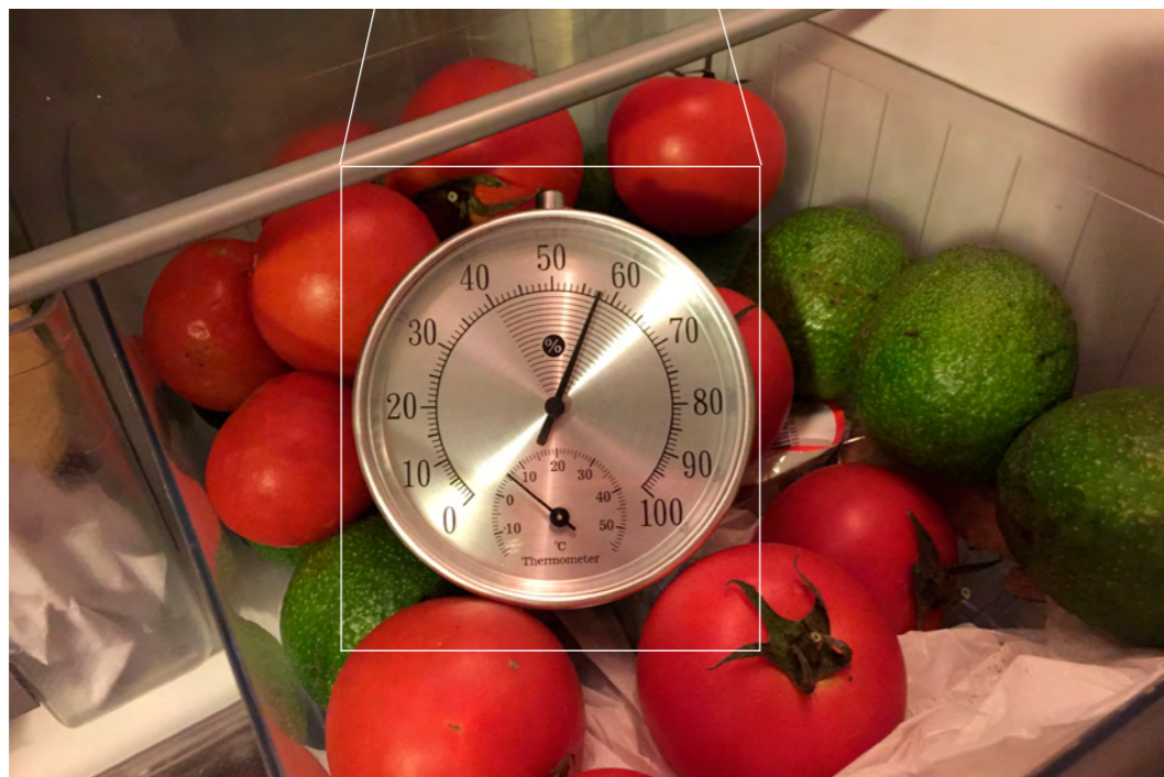
Fig.91 Measuring RH and temperature inside the 'crisper drawer' of Bosch Refrigerator Series 2.
