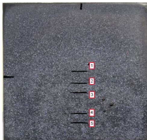
Figure 3.23 Micro etched billet sample 3490L1
