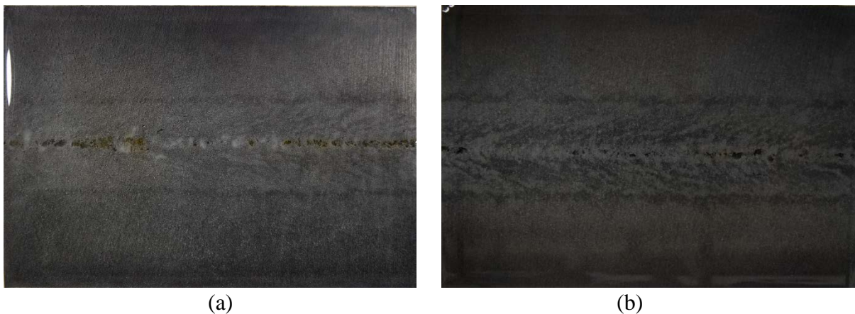
Figure 3.14 Central porosity in longitudinal section without final EMS (a) with final linear EMS
