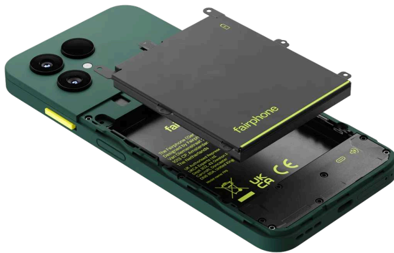
Figure 11. Fairphone back structure (Source: Fairphone official website, https://shop.fairphone.com (accessed in 2026))
