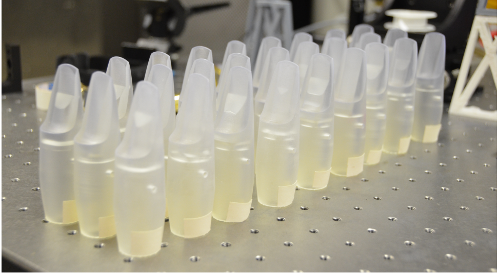
Figure 5.9: 27 different mouthpieces designs tested in the experiment.
