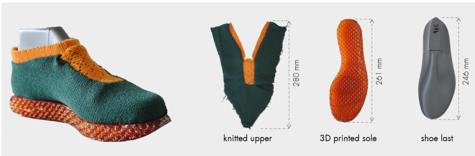
Figure 4.2: Prototype of knitted footwear with 3D-printed sole (size EU37B).
