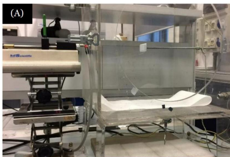
Figure 3.7. Electrospinning setup used in this work
