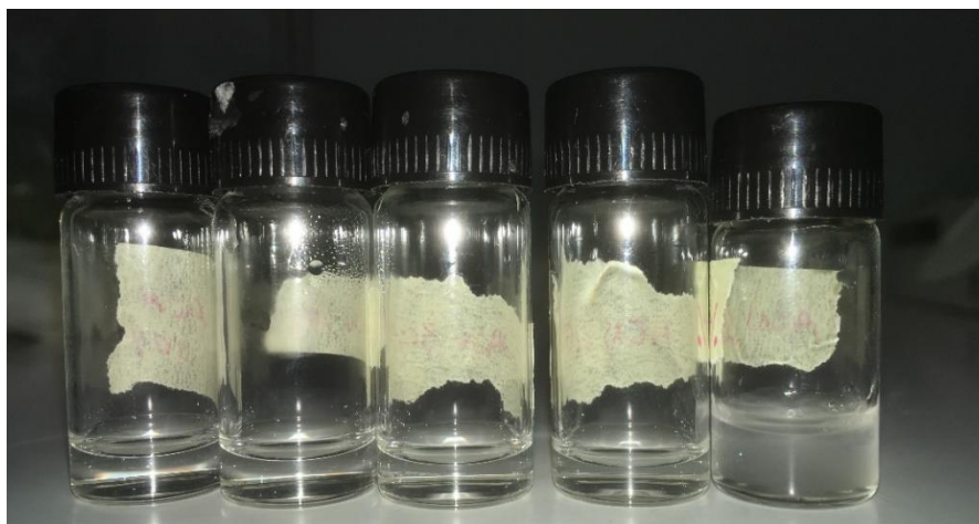
Figure 4.24 PVA in water-ACN blends, with ACN volume fraction of (from the left to the right): 10, 20, 30, 40, 45 %
