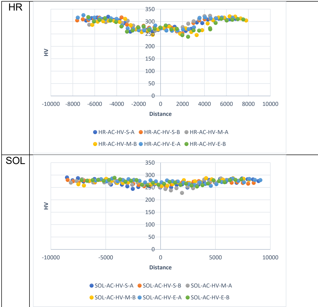
Figure 31 shows hardness variation with distance in TIG AC welding.
