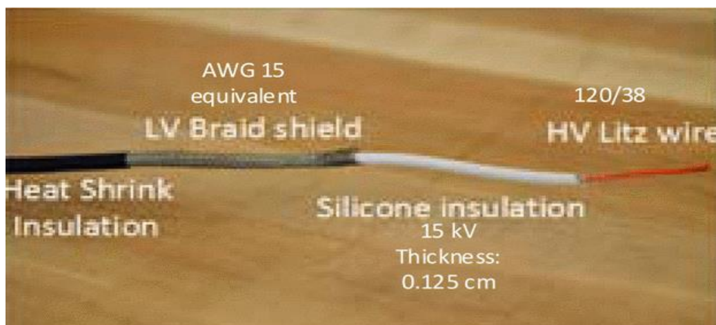
Figure 3.18 Structure of coaxial cable.
