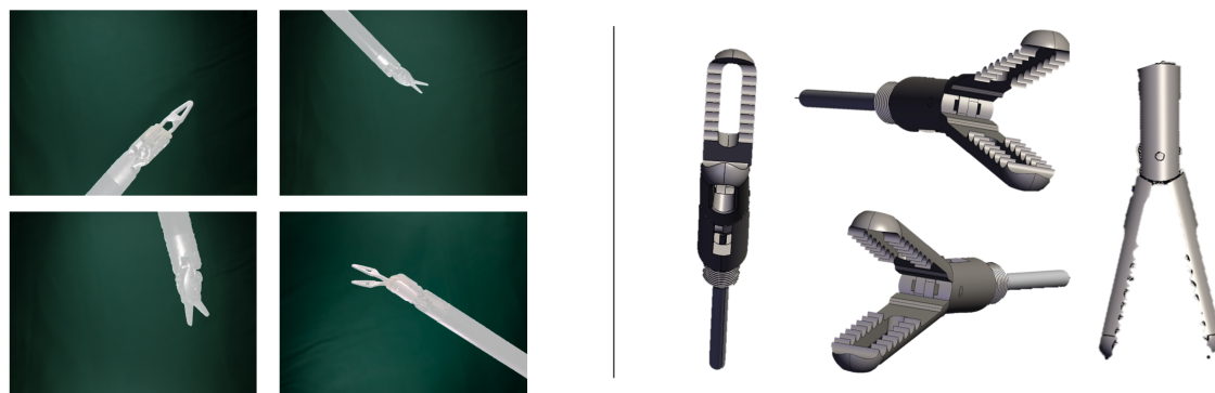
Figure 1.14: Left: shape-priors, in the form of binary segmentation masks of the instruments, obtained from automatic segmentation of chroma-key images. Courtesy of [GPHFD + 21]. Right: different views of a 3D CAD model of a laparoscopic forceps head. Courtesy of [Gra]
