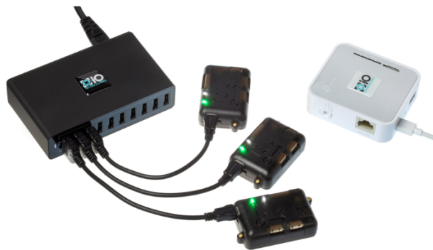
Figure 2: NGIMU sensors (x-io Technologies Limited Bristol UK, USB station for simultaneous charging of multiple IMUs and TP-link router ( TP-Link Corporation Limited) for wireless connection
