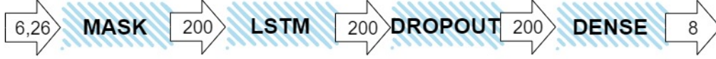
Figure 11: Schema of the sequential model built for primitive classification. The number in the arrows represents the dimensionality of the input/output vector for each layer. The ML model consists of four key components: a masking layer, a LSTM layer, a dropout layer, and a dense one.
