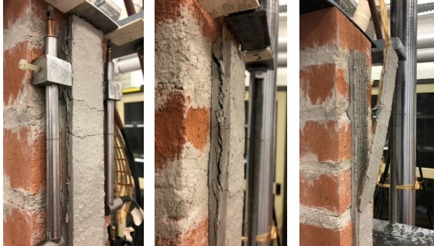
Figure 4-11: D_{mf} failure accompanied with macro cracks noticed on PBO FRCM of specimen DS_300_50_P_R_3
