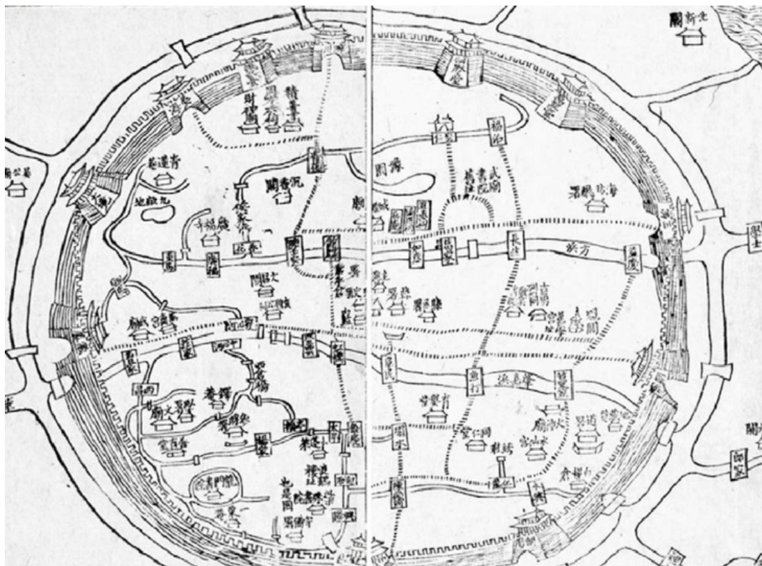
Figure 9: A plan of Shanghai walled city showing the basic traditional planning of a Chinese city.
