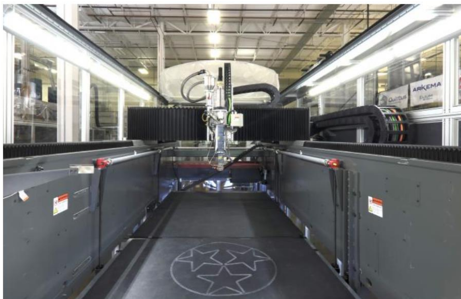
Figure 5: BAAM printer realized by Cincinnati Incorporated at Oak Ridge National Laboratories [4]
