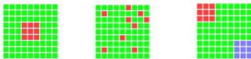
Figure 2: Examples of the three defective scenarios: single cluster (left), sparse defects (centre), two clusters (right)
