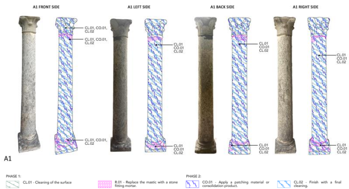
Figure 35: Restoration techniques mapping on a column of Chiostro della Memoria east façade
