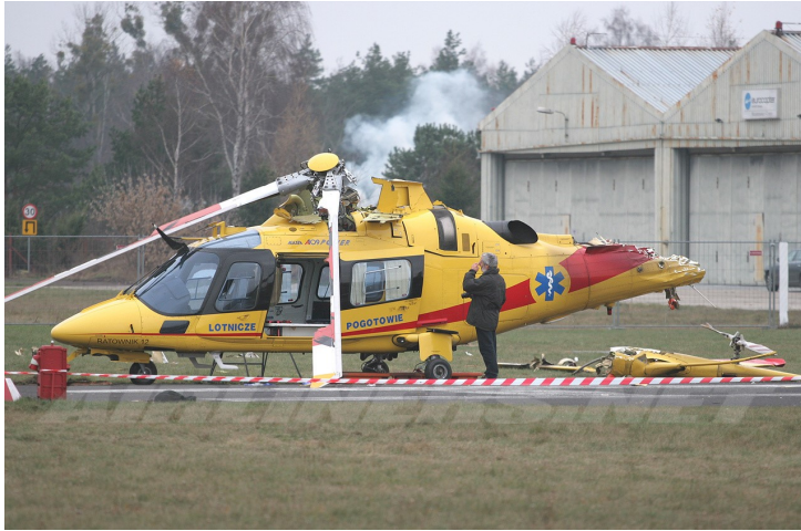
Figure 2: Accident of an AgustaWestland AW-109E probably due to ground resonance, Poland - November 21, 2009 , photo from Jakub Kalinowski.
