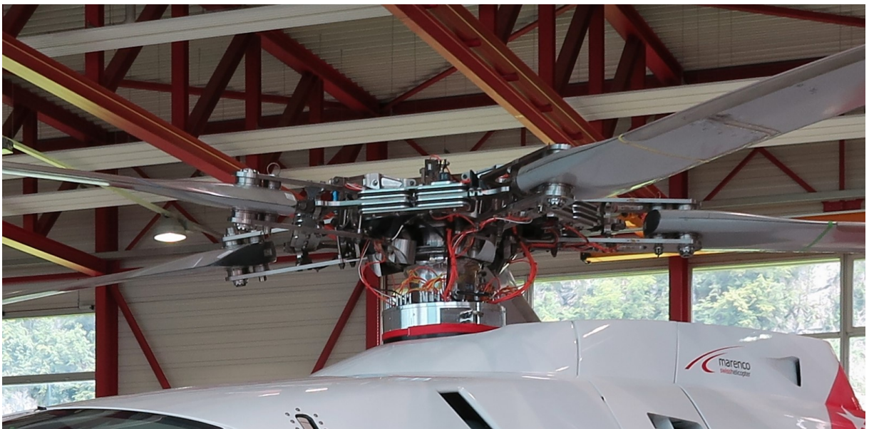
Figure 3.20: Rotor of the Kopter AW09, Inter-Blade configuration with an elastomeric damper.
