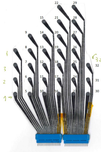
Figure 5: Maxine electrodes used for sEMG acquisitions: it is composed of 32 dry electrodes
