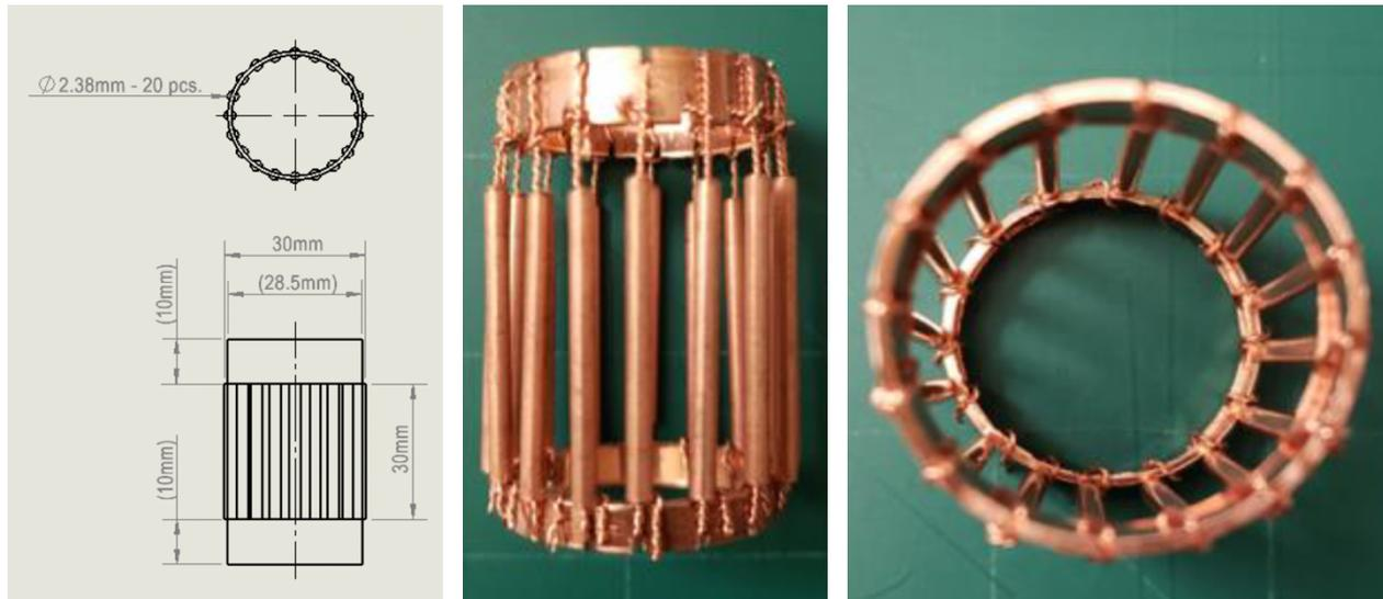
Fig 1.14 Cylindrical Fog Cage (CFC)
