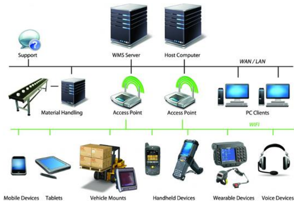
Figure 3 - Warehouse Management System Network
