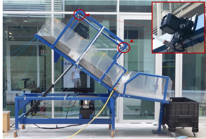
Figure 49: Action cameras position and prototype
