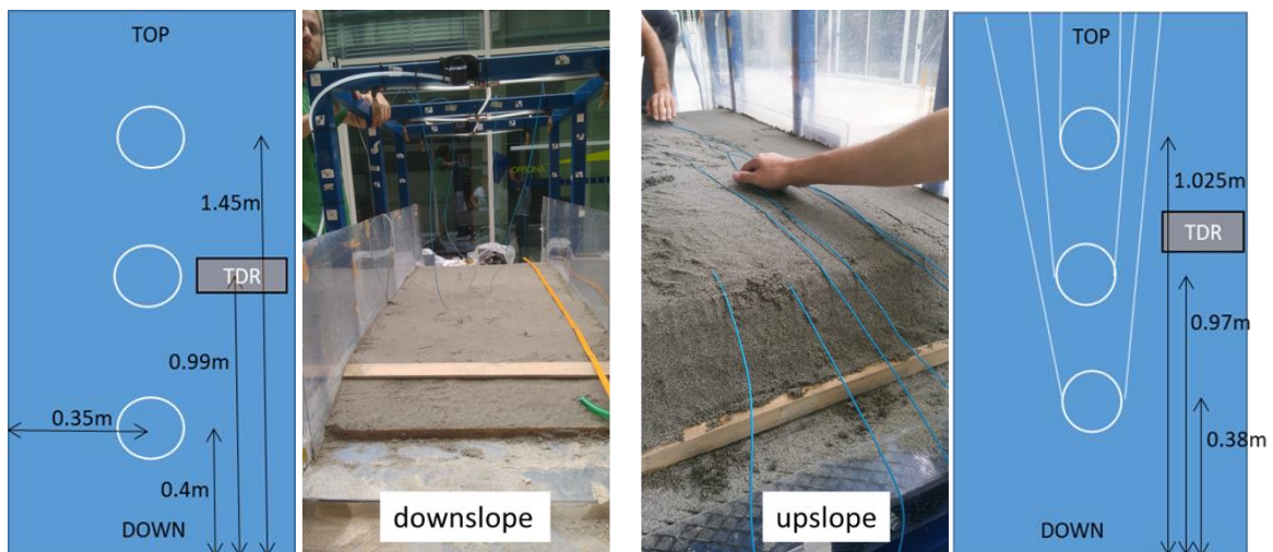
Figure 53: Types of FO cable installed configurations
