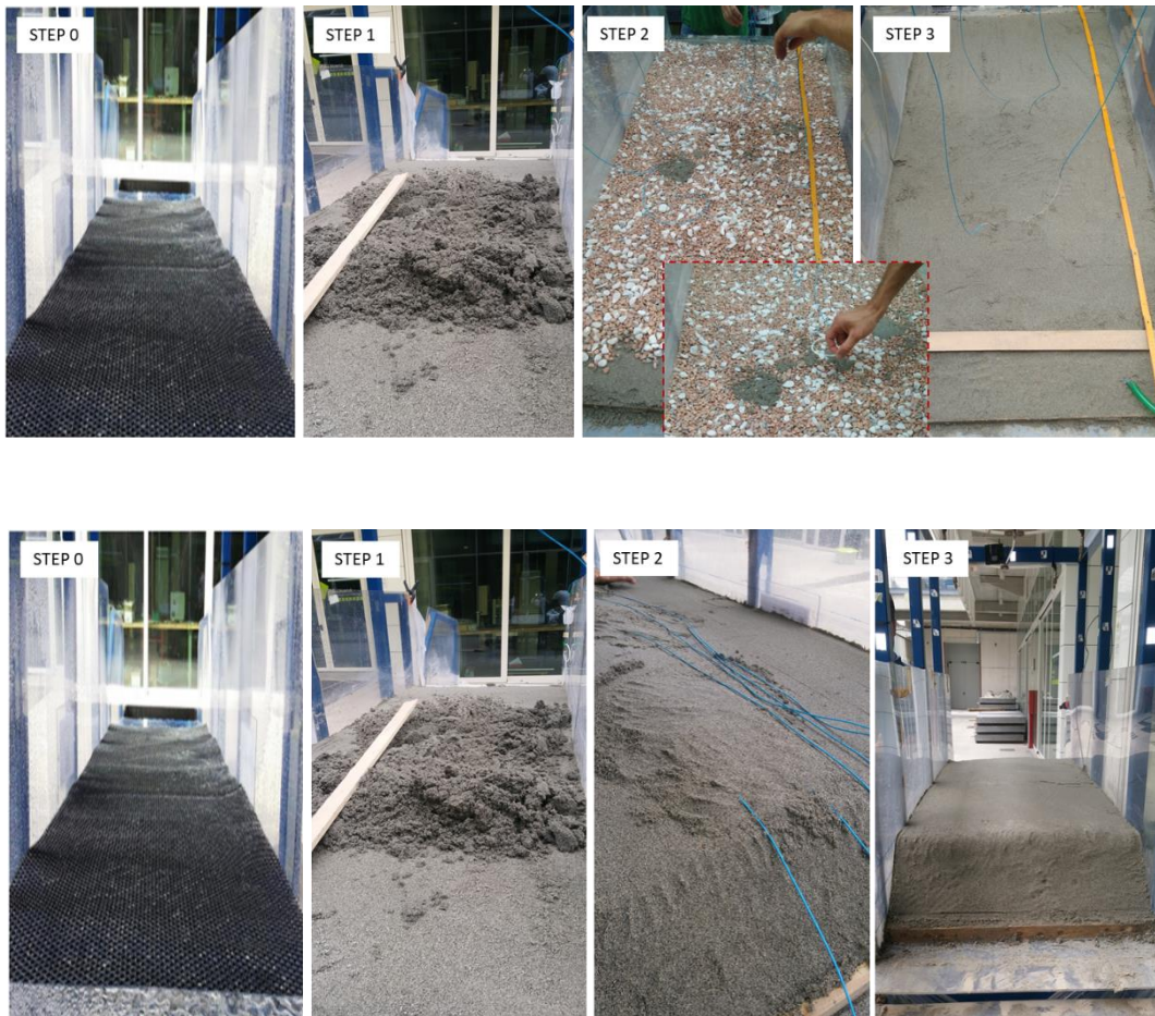
Figure 55: Steps for the preparation of the slope model in which different configurations for the fiber cables have been used: above the rest of the fiber cables protrudes out of the soil body surface, below the rest of the fiber cables cable leading out to the interrogating device runs within the soil and protrudes from the upstream end of the soil body.
