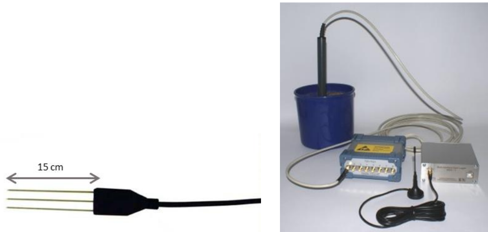
Figure 48: Three electrodes TDR probe and TDR system calibration
