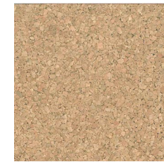
Cork Fibers Layer for Floor Acoustic and Thermal Insulation
