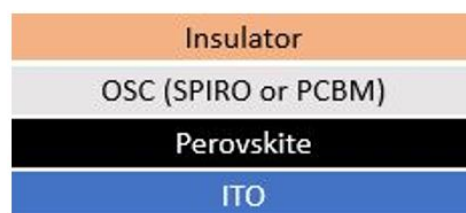
Figure 4.1. Schematic of the sample substrate.
