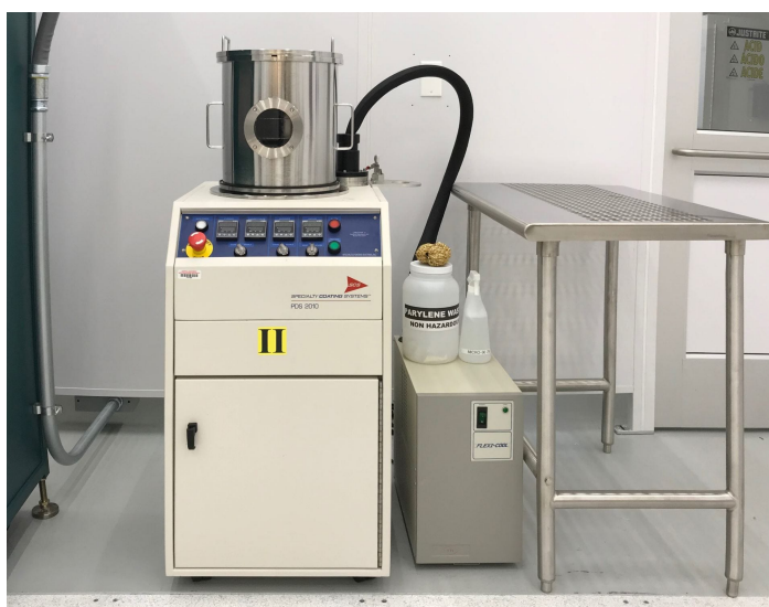
Figure 3.2. A picture of the parylene coater setup.
