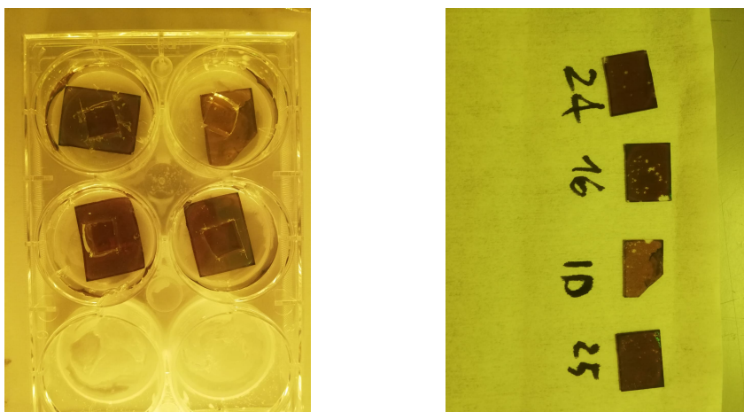
Figure 4.3. Couple of images taken during the water resistance test. On the left, a picture taken after samples been merged with water for an hour. On the right, the samples are shown after 4 hours of direct contact with water.
