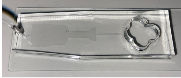
Figure 2-1: PDMS microfluidic device fabricated via soft lithography and bonded to a glass slide. An inlet tube allows fluid injection into the channel, and a collection well at the outlet retains the expelled gel and fluid.
