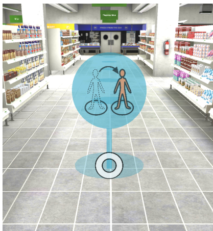
Figure 5.7. Camera UI pointer centered on the interactive object. It is bigger than default to inform user that they are pointing an interactive object.
